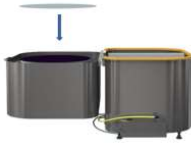
Figure 3.22: Inserting silicon wafer to the spray coater
