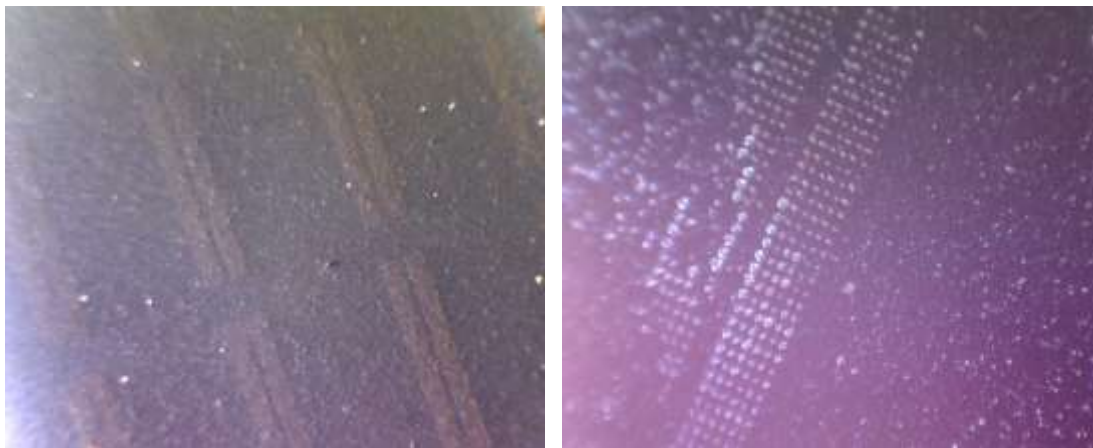
Figure 4.22: magnified images of silicon wafer coated by spray head model two
