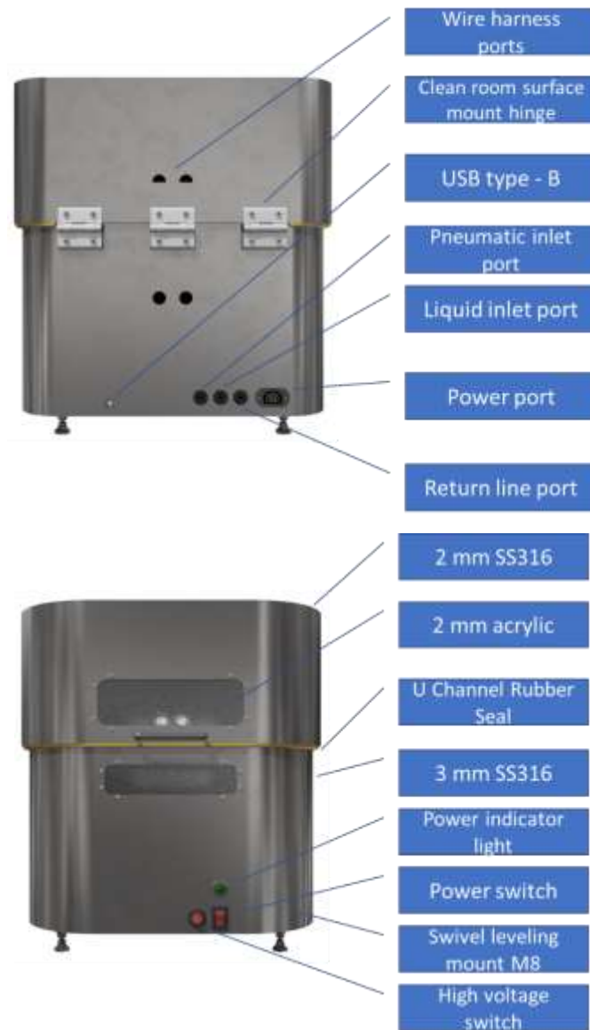
Figure 4.14: Enclosure with naming all the parts
