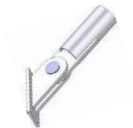
Figure 3.13 Concept of knee brace connection
