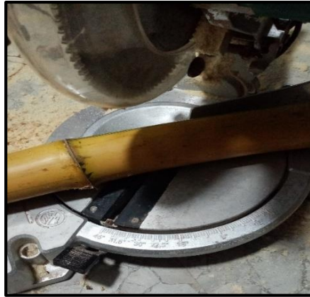
Figure 3-4: Preparation of Bamboo structures using Circular power saw.
