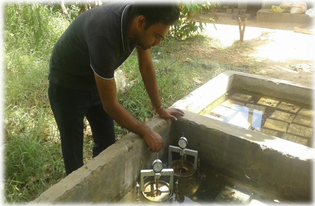
Figure 44: CBR swell observation under the 4 days soaked condition
