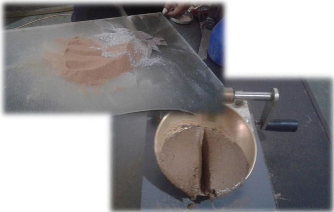
Figure 33: Atterberg limit laboratory test for PHA composite sample
