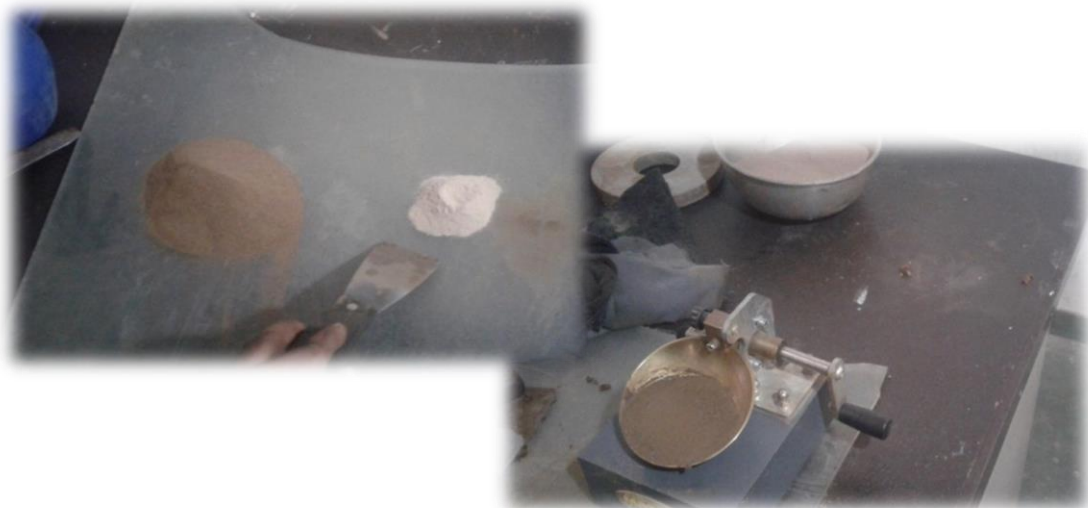
Figure 25: Preparation for glass composite sample for Atterberg limit test
