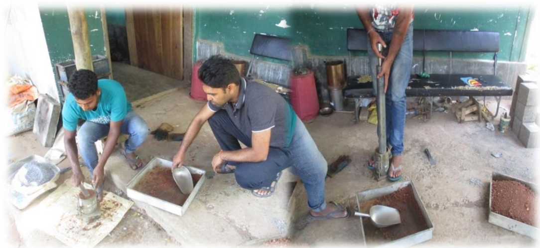
Figure 40: Preparation of PHA Composite Sample for Proctor Compaction Laboratory Testing
