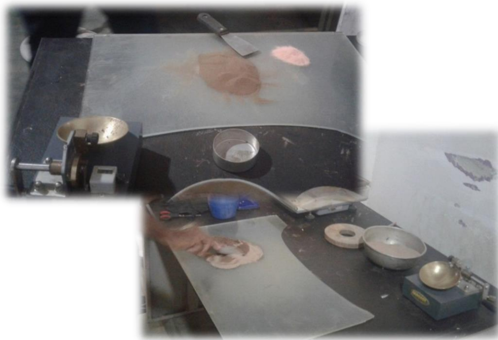
Figure 29: Atterberg limit test for plastic composite sample
