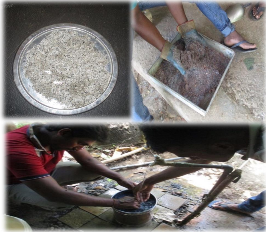
Figure 38: Laboratory Sieve analysis test composite sample preparation for PHA composite sample
