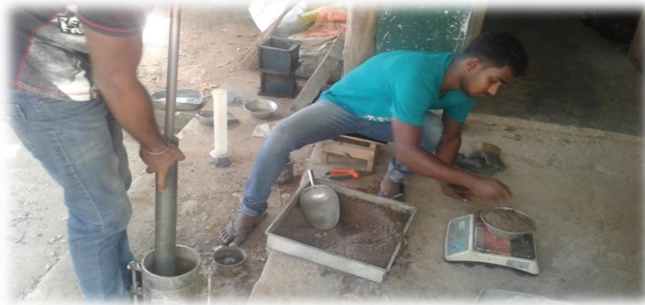
Figure 42: Preparation of PHA composite sample for CBR laboratory testing
