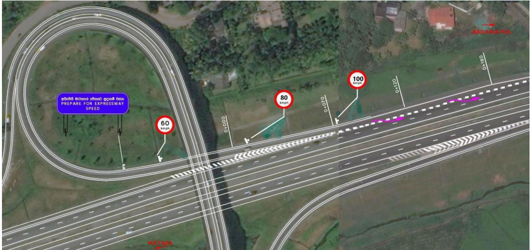
Figure 5.1 Proposed Sign Board Arrangement at Kottawa Interchange
