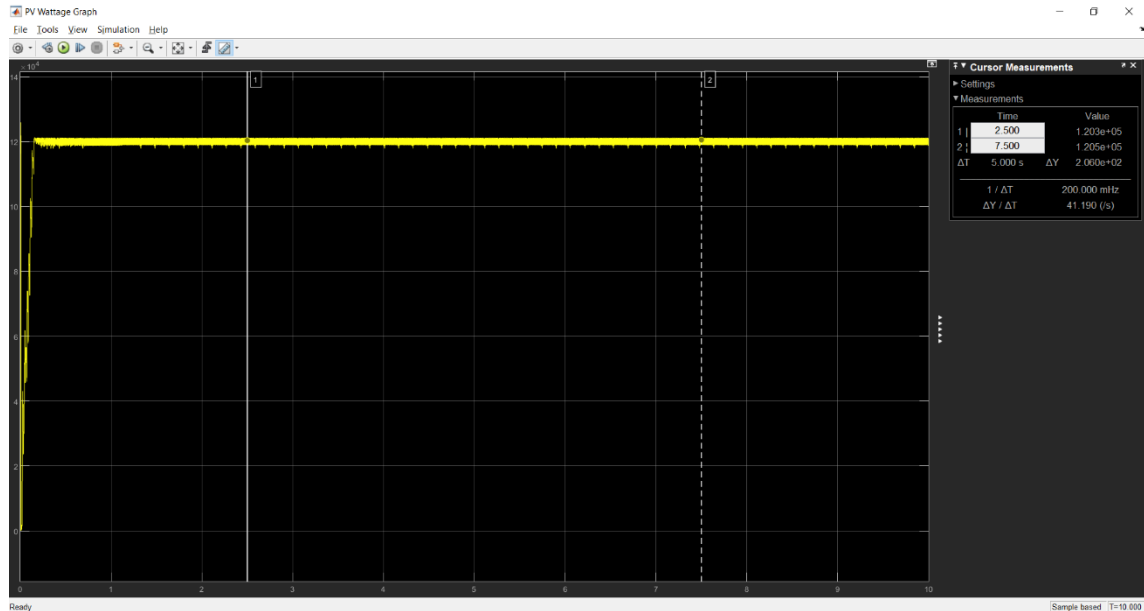
Figure 7.26: Fluctuation of wattage in conventional MPPT at Temp.30°C & Irr. Level 1,250 W/m 2 .
