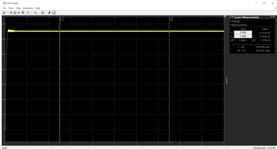
Figure 7.12: Fluctuation of voltage reference in conventional MPPT at STC.
