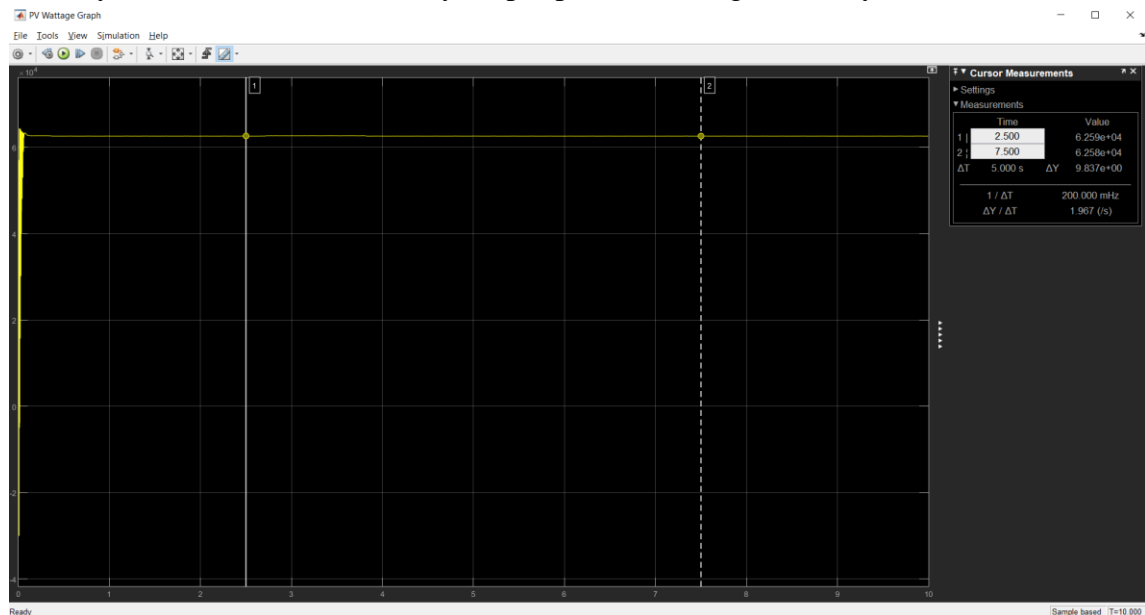
Figure 7.19: Wattage in VCIT-MPPT at Temp.15 °C & Irr. Level 600 W/m 2 .
