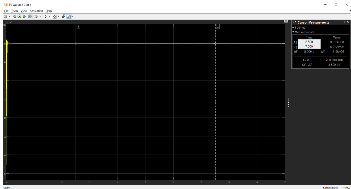
Figure 7.21: Wattage in VCIT-MPPT at Temp.20°C & Irr. Level 800 W/m 2 .
