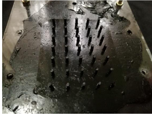
Figure 7.13: Polymer layer with excess material parts.
