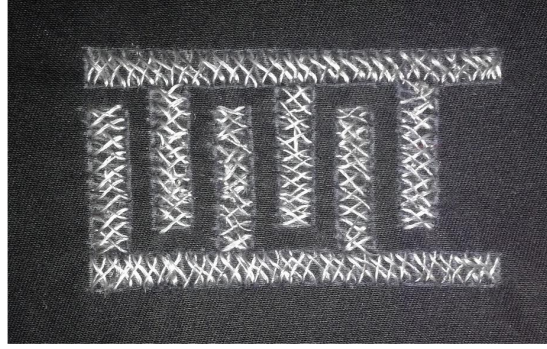
Figure 7.7: Electrodes were sewn by hand using cross-stitches.
