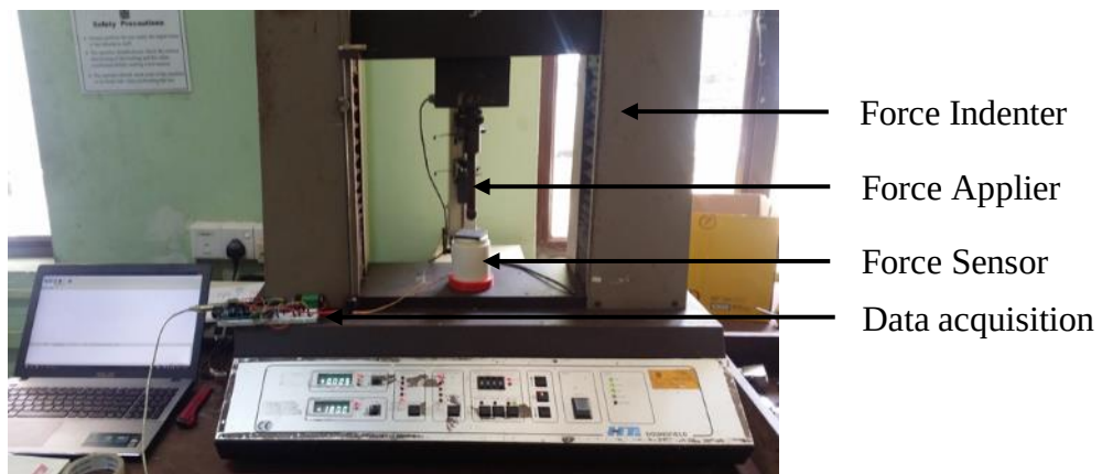
Figure 5.23: Force indenter was used to conduct experiments.
