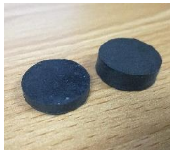
Figure 3.12: Fabricated sensing elements with different thicknesses.
