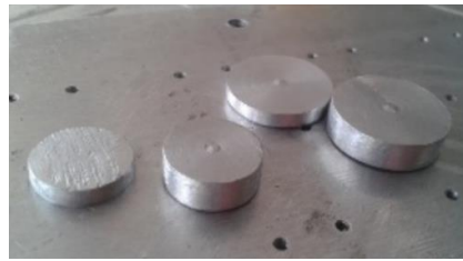
Figure 3.11: Spacers fabricated to adjust the thickness of conductive polymer samples.
