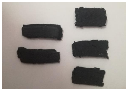
Figure 4.10: Transversely sectioned conductive polymer samples.
