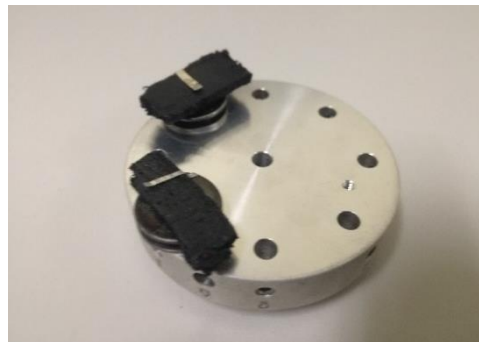
Figure 4.12: Prepared samples were placed on SEM studs.
