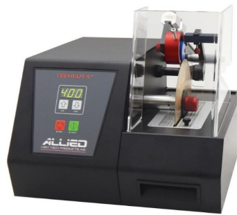
Figure 4.9: Low speed saw with a diamond cutter was used.
