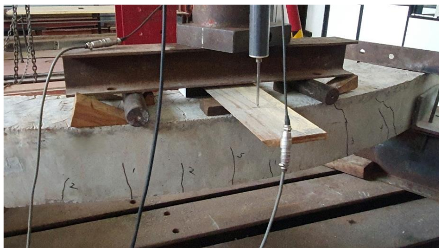
Figure 22: Cracks in a Beam 1-2-CO
