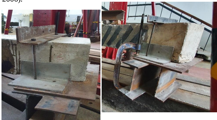
Figure 17: 4 sides clamped at supports
