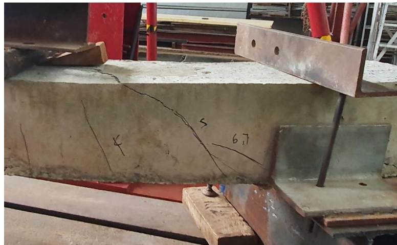
Figure 20: Shear + Torsional failure of Beam 1-1-CO
