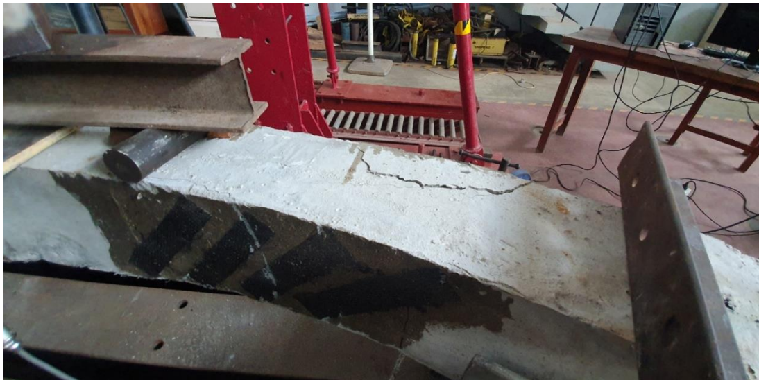
Figure 31: Cracks in a Beam 2-1-SS
