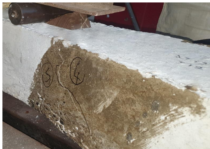
Figure 26: Shear failure of Beam 2-1-FS
