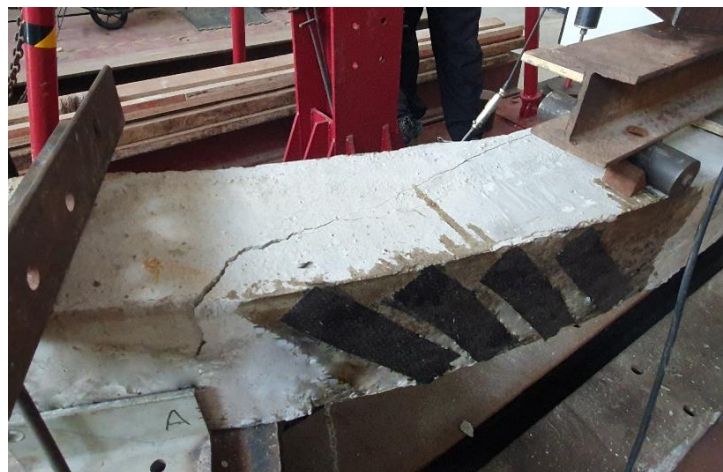
Figure 32: Torsional failure of Beam 2-1-SS
