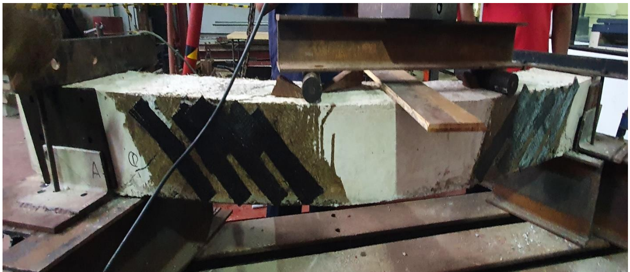
Figure 35: Cracks propagation at CFRP zone in Beam 2-2-SS
