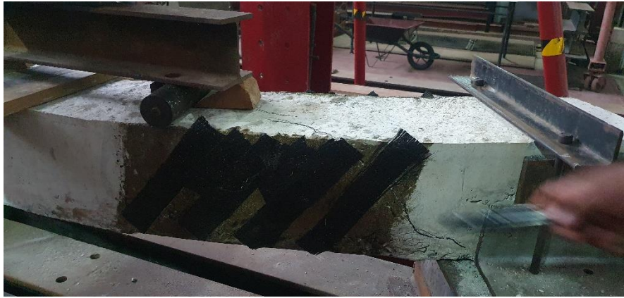
Figure 34: Cracks in a Beam 2-2-SS
