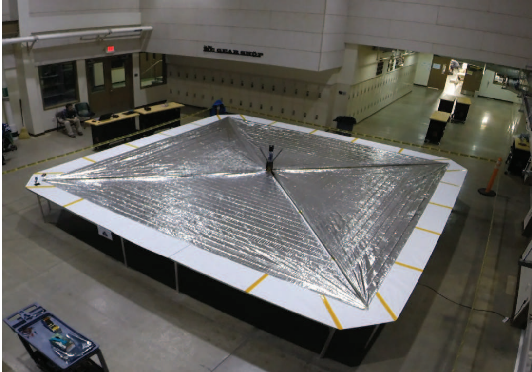
Figure 1.3: LightSail-2 spacecraft sitting on its low friction deployment table following a successful solar sail deployment test at Cal Poly San Luis Obispo on January 28, 2016
