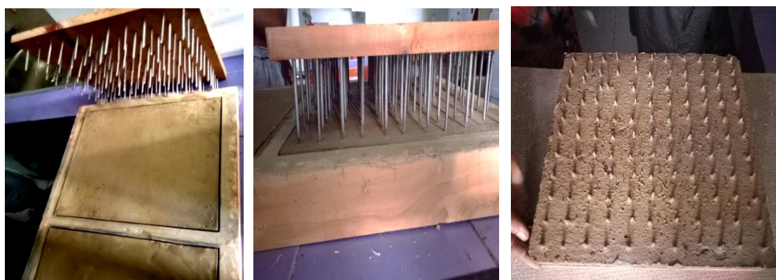
Figure 4-11: Clay samples compressed by hand in timber frame and pounced with a nail plate into a regular pouncing pattern
