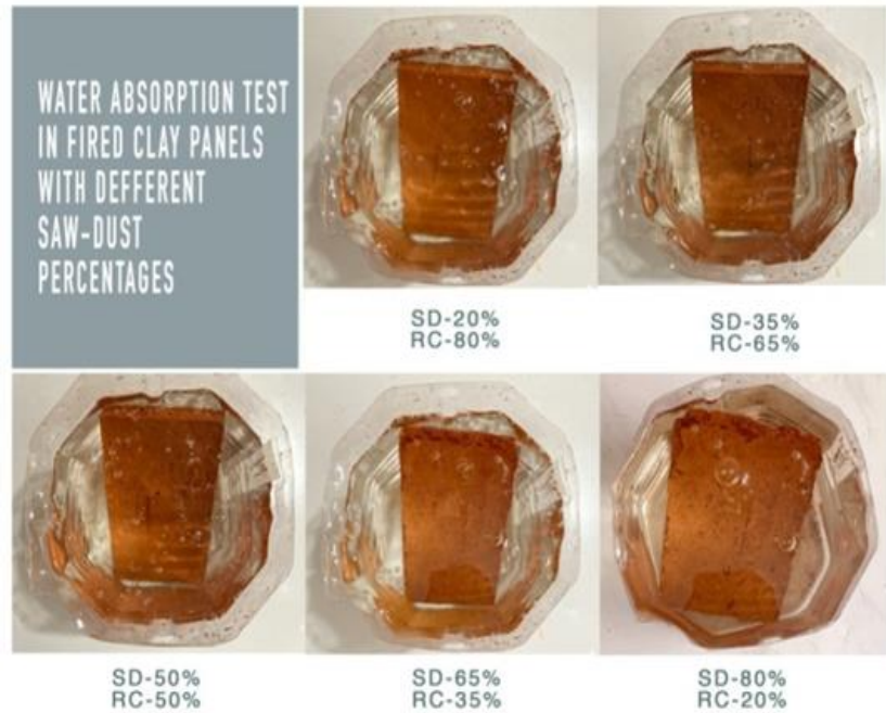
Figure 3-17: Testing the water absorption - red clay panels with different compositions of Saw dust
