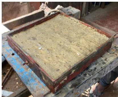
Punching the compressed clay panel
