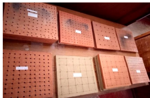
Figure 4-13: Punched and fired clay panels, the final product
