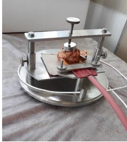
Figure 3-24: Testing the thermal conductivity of the DCDW specimen with Transient Hot Bridge - Thermal Conductivity Meter
