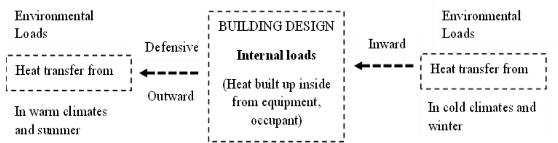
Figure 1-2: Bio-Climatic Design to moderate between climate and building interior for cooling thermal loads, defensive outward heat transfer in summers and inward promoting heat transfer in winters.
