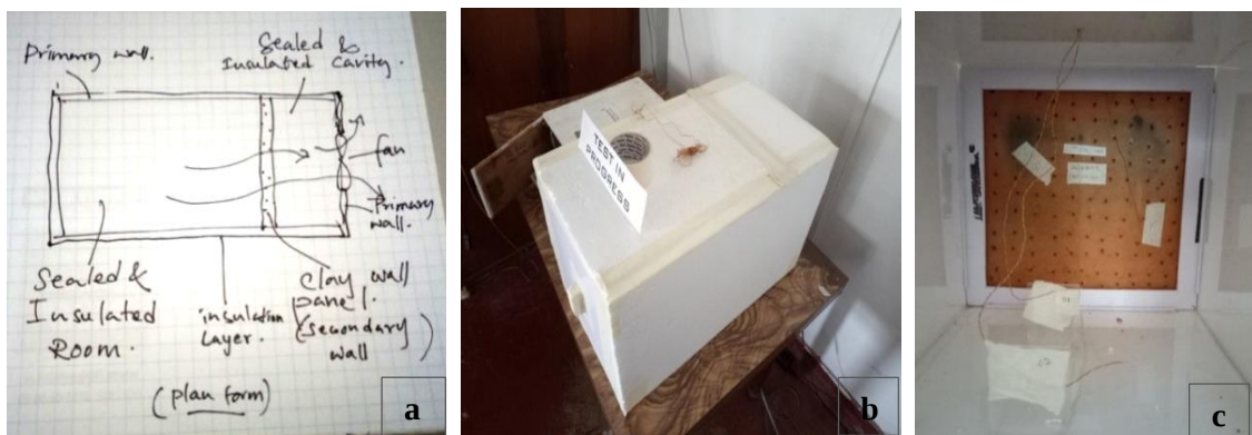
Figure 4-15: During the Chamber Test; Investigating the Indoor air temperature reduction a) Sketch plan form of the test chamber. b) Insulated outer look of the test chamber. c) DCSW panel is installed to the test chamber and ready to investigate the thermal performance
