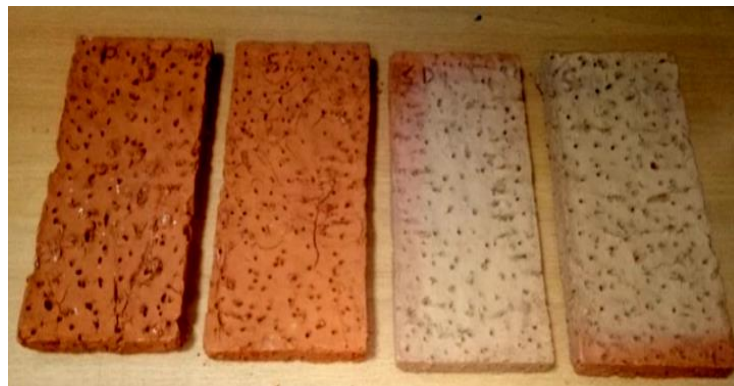
Figure 4-9: Specimens made for pilot casting; compressed by hand in timber frame, punched randomly with a nail and fired to 800°C for 60 min.
