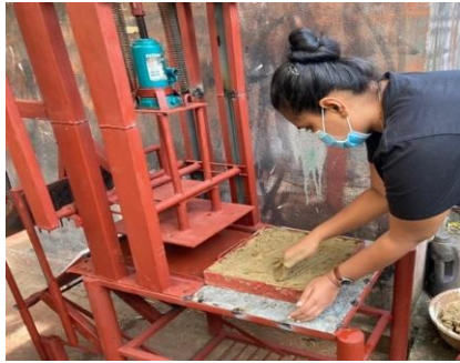
Clay lump is loaded in the steel frame
