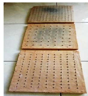
Figure 4-13: Punched and fired clay panels, the final product
