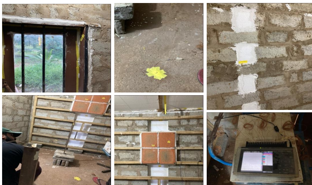
Figure 5-15: Measuring the indoor temperature reduction; Locating the thermal probes to capture the temperatures for 24 hours, for each identified case
