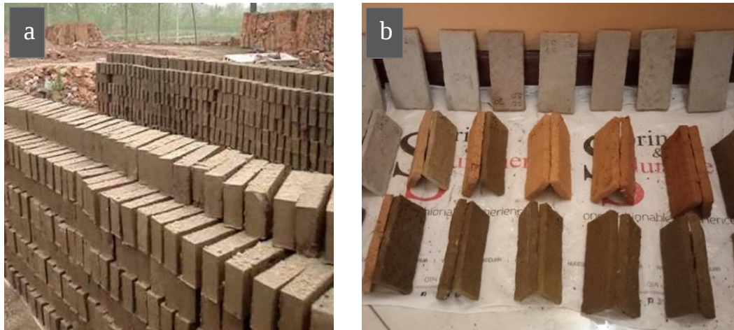
Figure 3-5: Traditional method of air drying the clay bricks.
