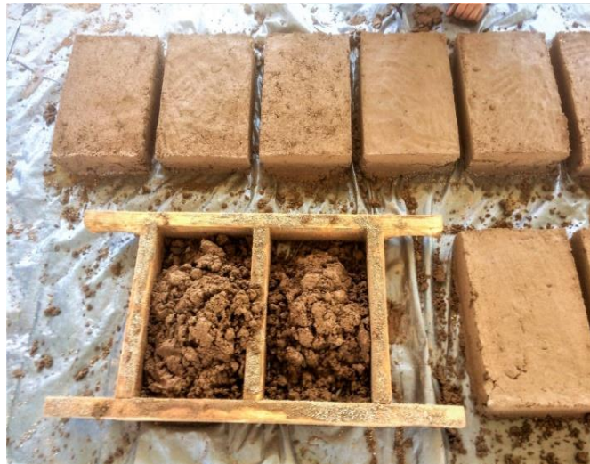
Figure 3-4: Traditional method of casting clay bricks manually, using timber mold
