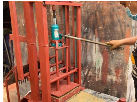
The clay lump is compressed manually with hydraulic power.
