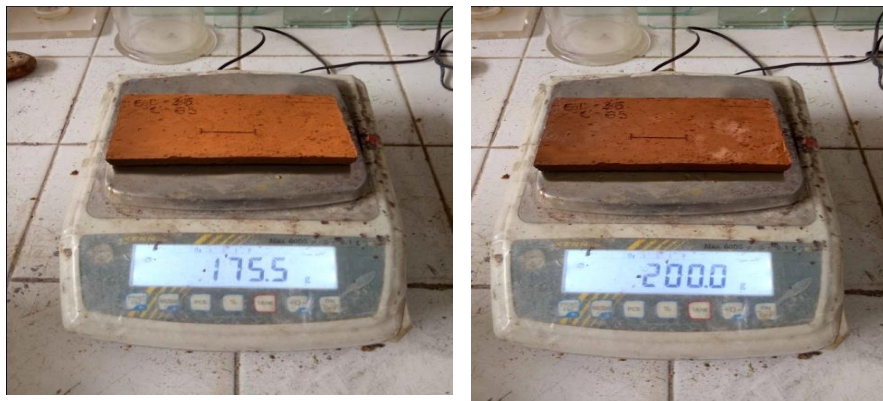
Figure 3-13: Letting the samples for water absorption and weighting before and after soaking
