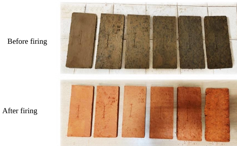
Figure 3-28: Red clay samples with five different Saw Dust compositions and with no compounds, Before and After Firing to 800°C
