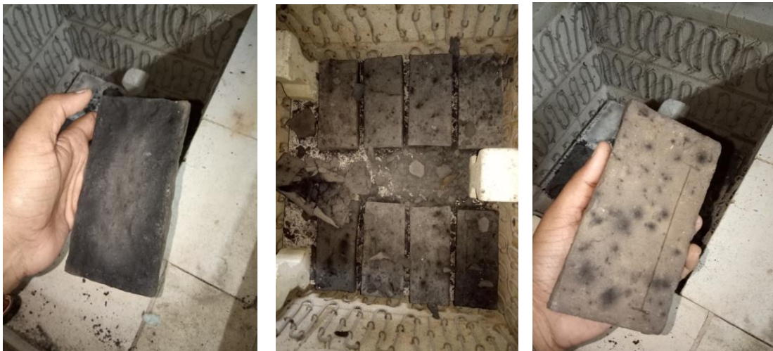
Figure 3-9: Samples fired to 400 C were either crashed, discolored, or cracked.
