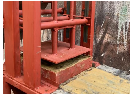
Steel frame loaded with clay is placed under the compression surface.
