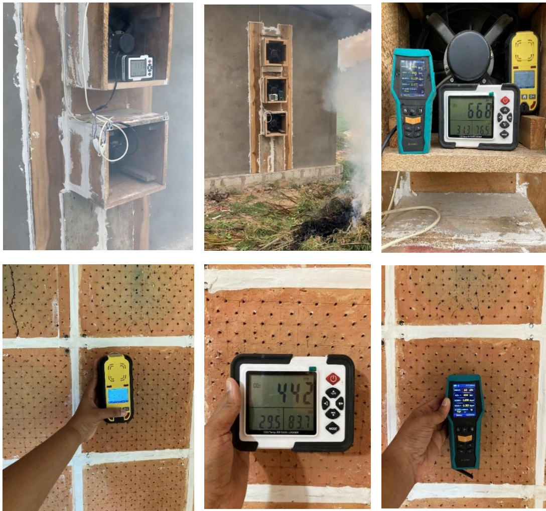
Figure 5-22: Data collection for air filtration capacity test
