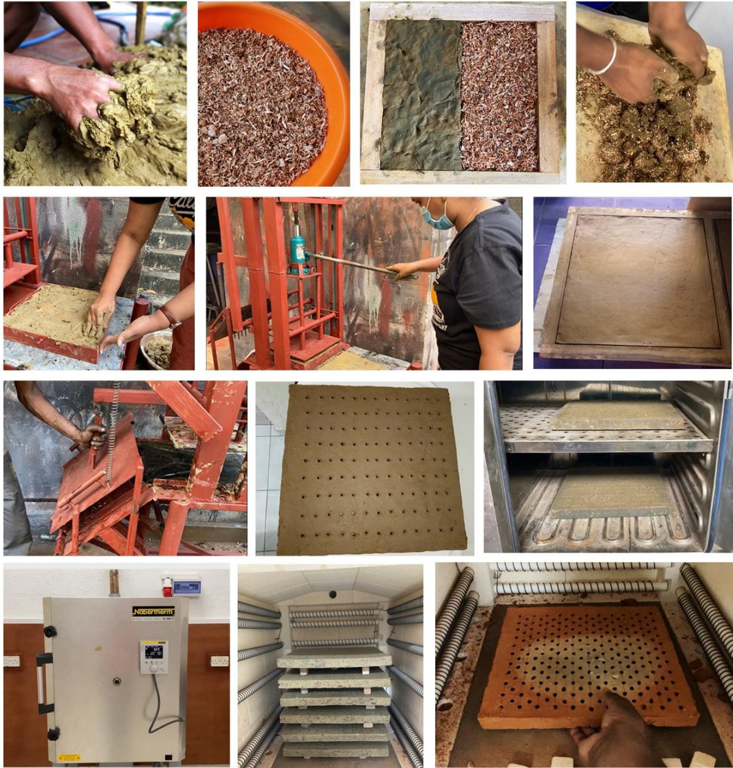
Figure 5-5: The casting process of DCDW panel; Raw materials, material mixing, compressing, punching, drying, and firing
