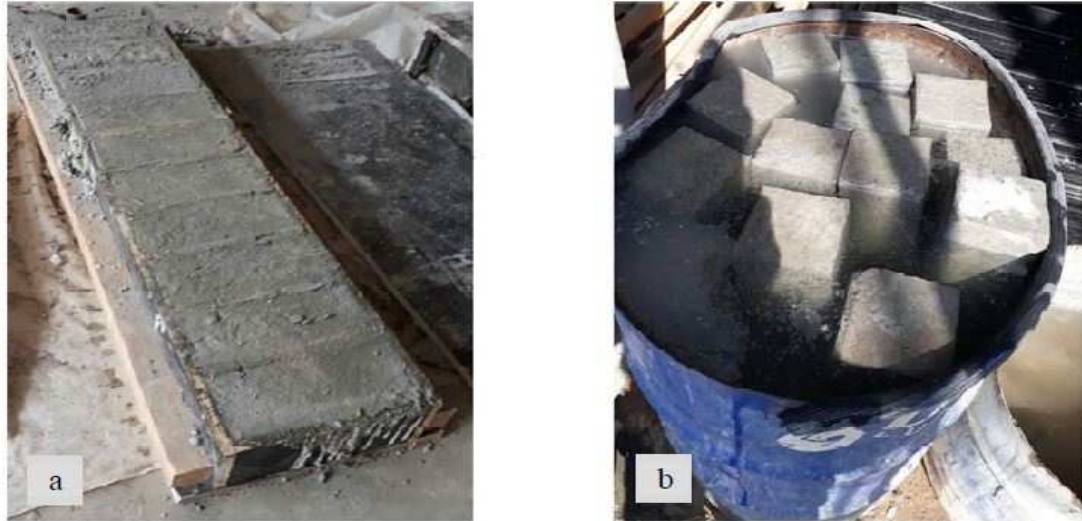
Figure 8. a) Grade 30 ready mixed concrete poured to moulds, prepared using coated plywood concrete blocks, and b) Immersed in water for 28 days for curing
