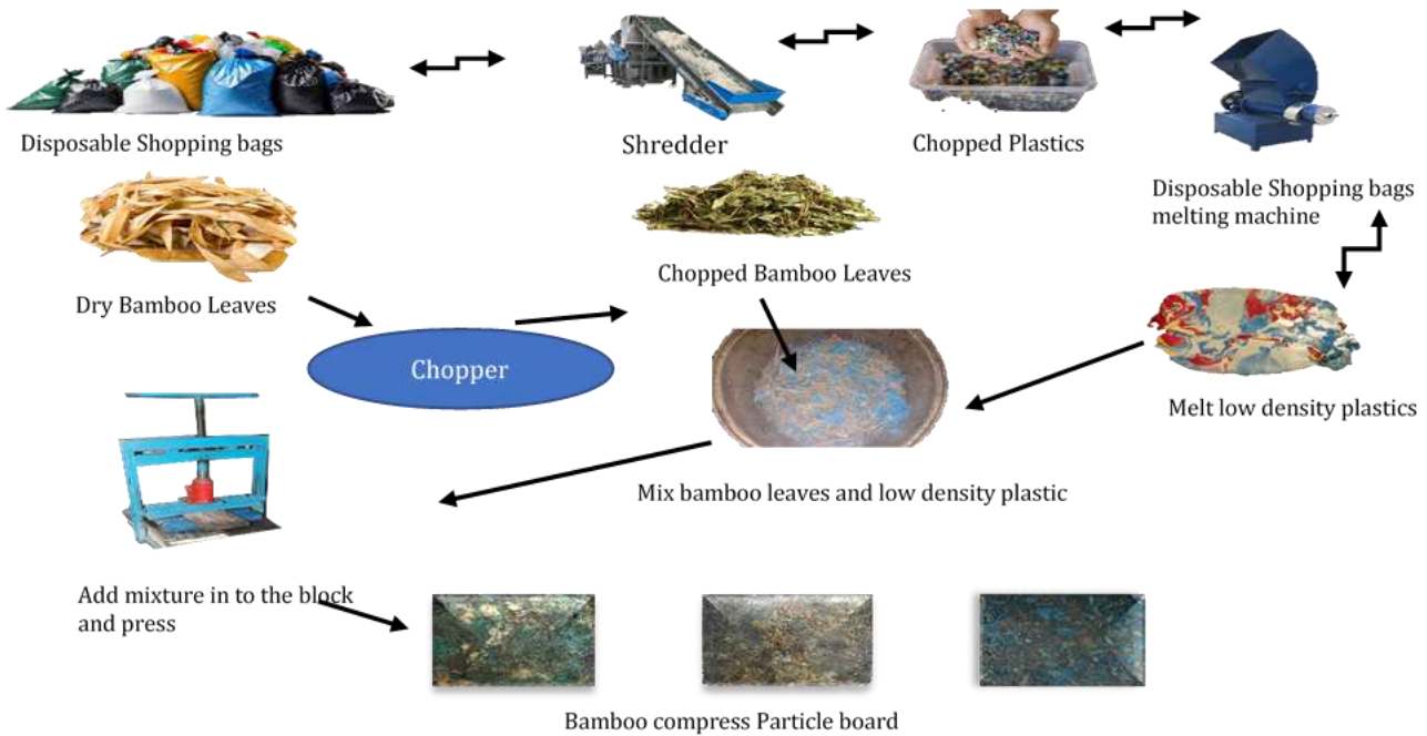
Flow chart 4: this chart shows the process of manufacturing dry bamboo leaves particle boards
