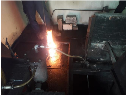
Figure 24-Starting the ignition using a burning piece of cloth
