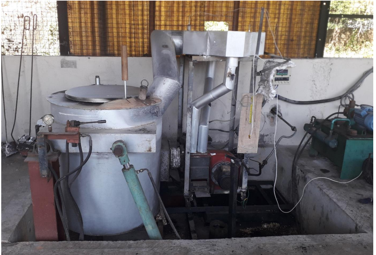
Figure 55-Integrated assembly of welded plate heat exchanger and the tilted crucible furnace consisting all the instrumentation for testing
