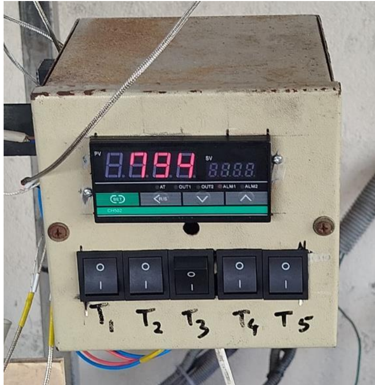
Figure 57-Digital temperature controller for temperature measurement, 1) T1-Cold air inlet, 2) Hot air outlet, 3) T3-Hot gas inlet, 4) T4-Hot gas outlet, 5) For temperature measurements inside the liquid aluminum
