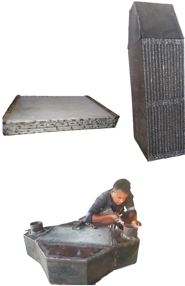
Figure 54-Fabricaiton of the welded plate heat exchanger
