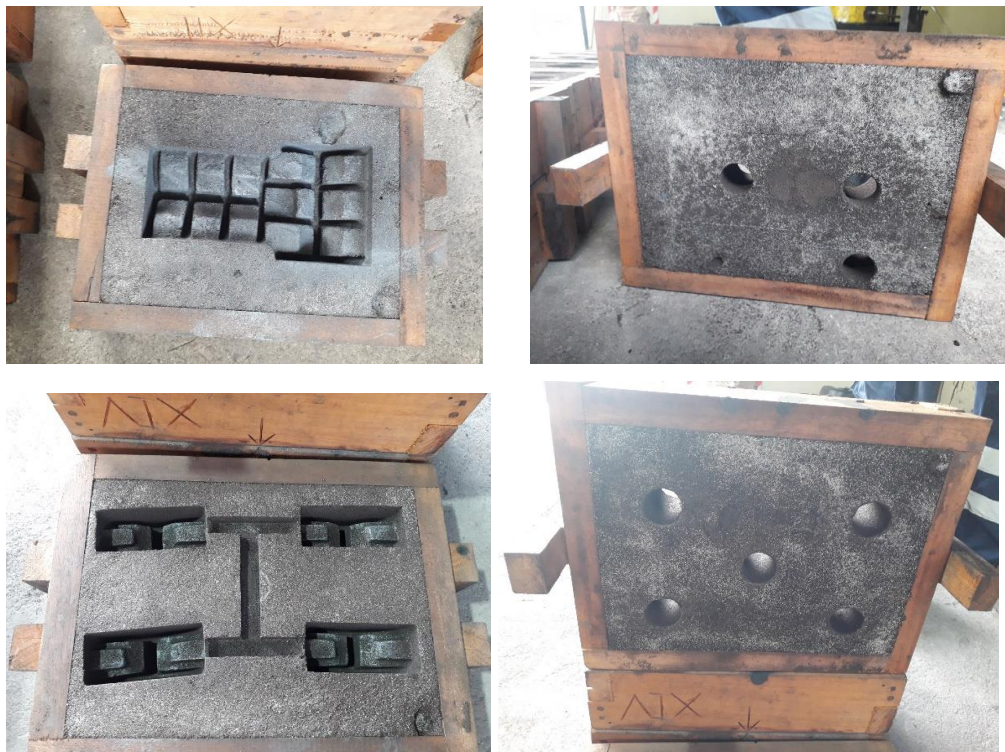
Figure 23-Sand cast mould ready for pouring
