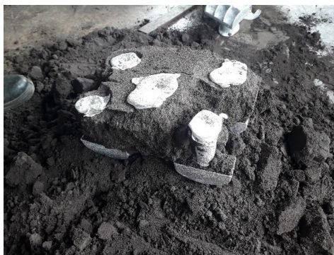
Figure 30-Pouring, Cooling and knocked out castings
