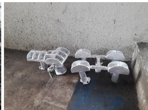
Figure 30-Pouring, Cooling and knocked out castings
