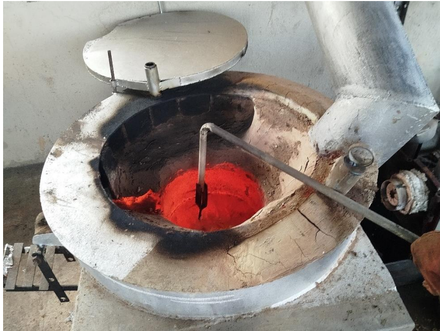
Figure 56-Molten aluminum temperature measurement using a K-type thermocouple
