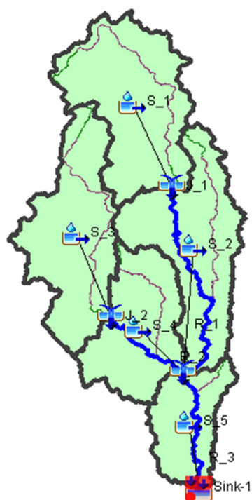
Figure 3-44 Catchment, sub-catchments, reaches, and streams delineated in HEC-HMS development
