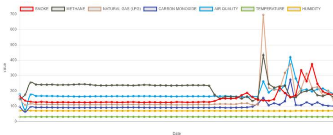
Fig.43. All Sensors Data Graph in Unstable Environment – thingspeak interface
