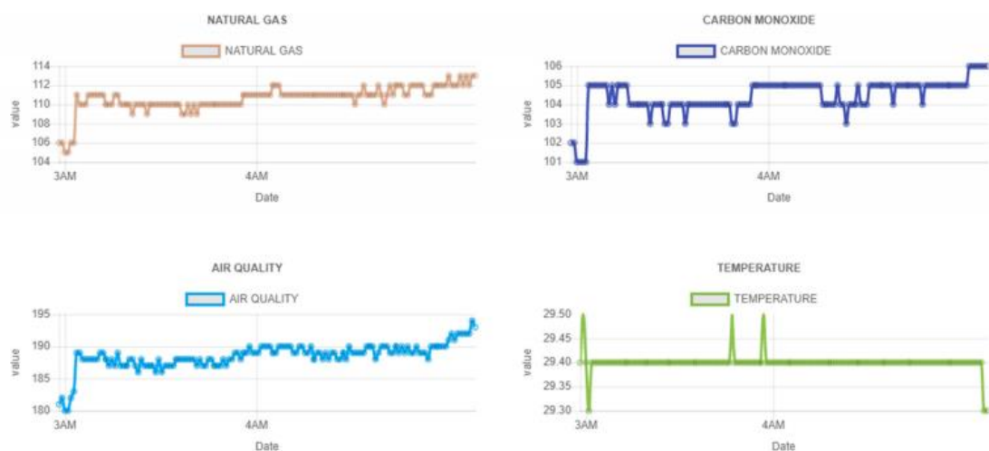
Fig.42. Data to Graph Visualization Natural Gas & CO Gas Vs Air Quality & Temperature-thingspeak interface
