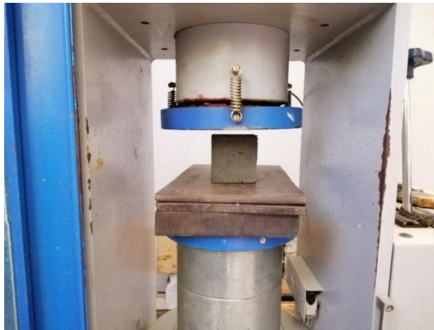
Figure 3.9: Test for compressive strength
