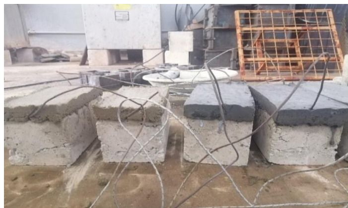
Figure 8.3: Specimens with thermocouples
