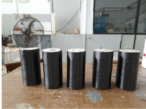
Figure 8.8: Concrete cylinder wrapped with CFRP layer
