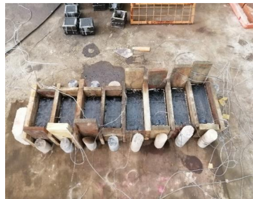
Figure 8.2: CFRP blocks with plaster
