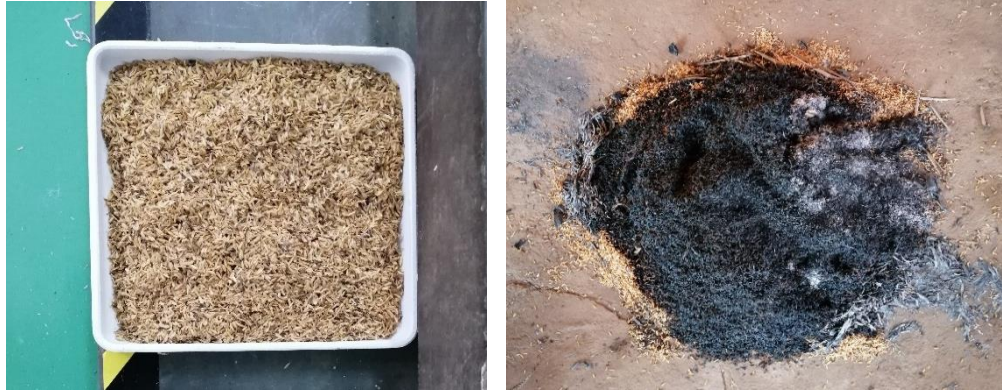
Figure 4.13: Raw rice husk before and after burning
