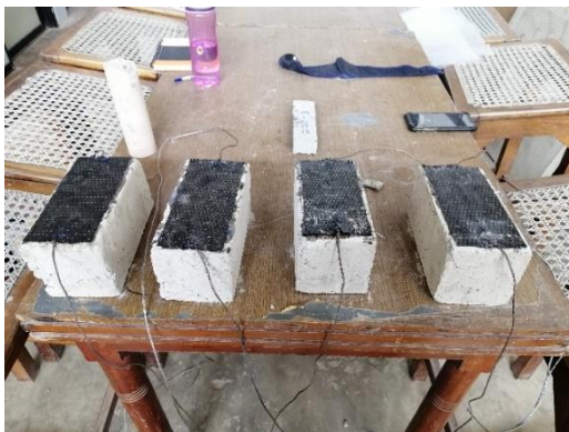
Figure 8.1: CFRP sheets with cement block
