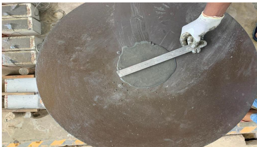
Figure 3.8: Flow of the mix
