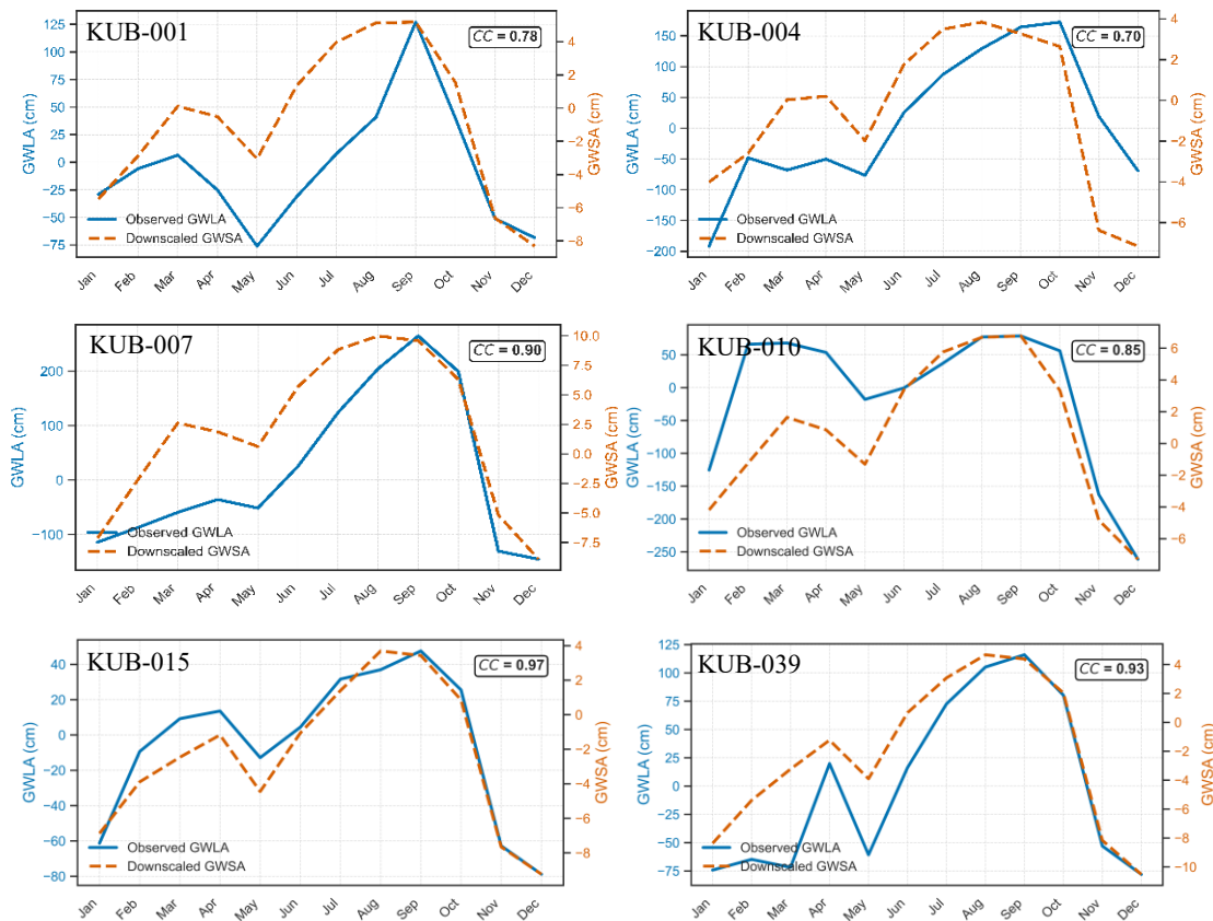
Figure 5-19: Time series plots compare long term monthly average in situ groundwater level anomalies (GWLA; blue line, primary axis) with downscaled groundwater storage anomalies (GWSA; orange line, secondary axis) at each well location across the basin
