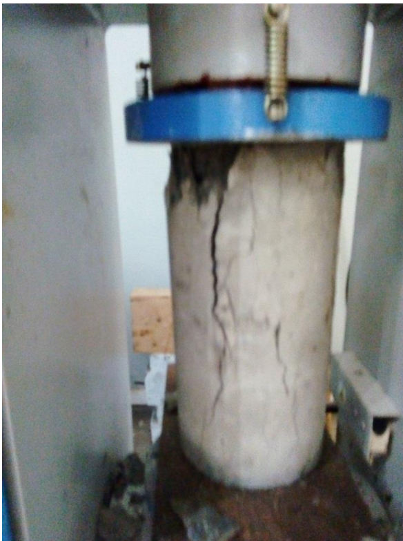
Figure 4.3.6 – Compression Testing Machine with Crushed Specimen
