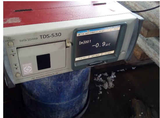
Figure 5.1.4 – Observation of readings from data logger before stressing the strands.
