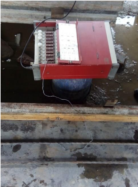
Figure 5.1.3 – Data logger connected to electronic strain gauge.
