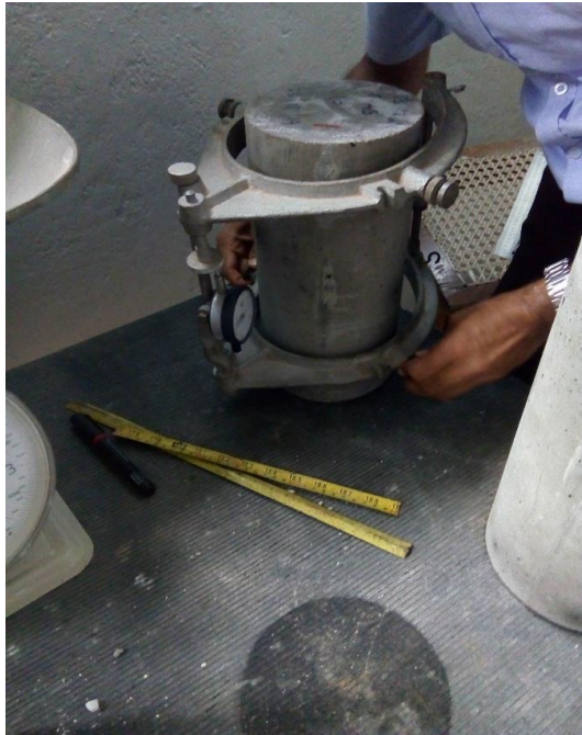
Figure 4.3.2 – Prepared concrete cylinder specimen for testing
