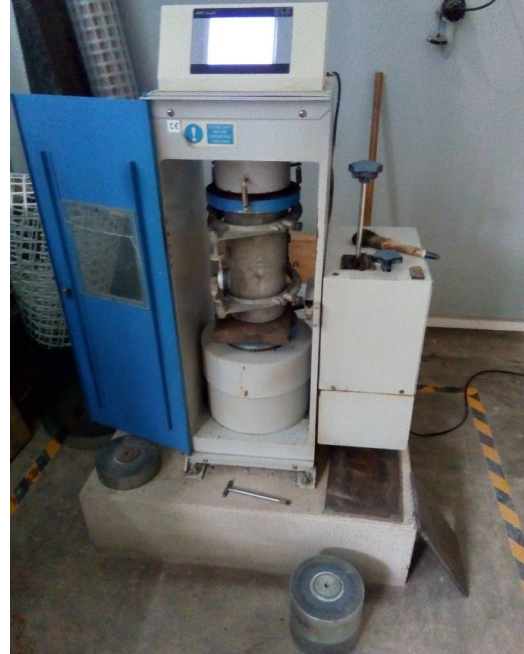
Figure 4.3.3 – Compression testing machine with Specimen placed in
