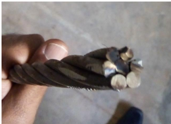
Figure 4.2.3 – Cross section of prestressing strand.
