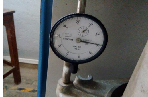
Figure 4.3.5 – Dial gauge connected to concrete cylinder specimen
