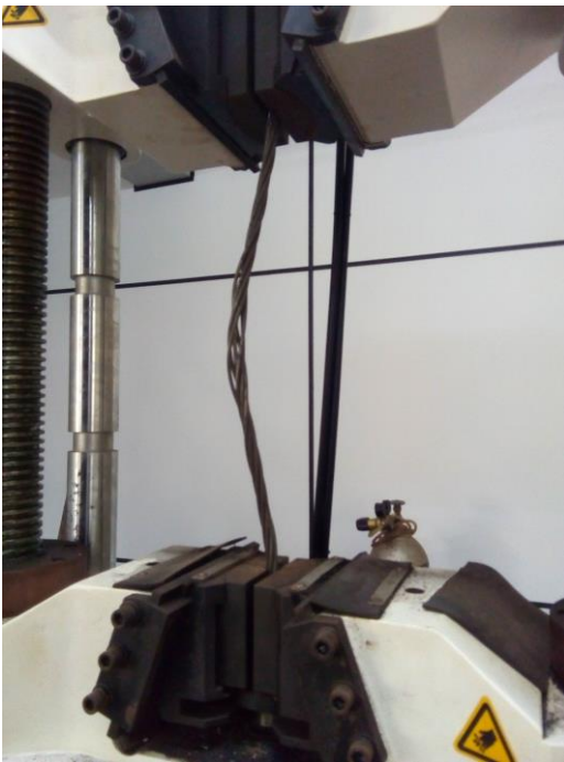
Figure 4.2.6 – Failure of prestress strand during tensile testing
