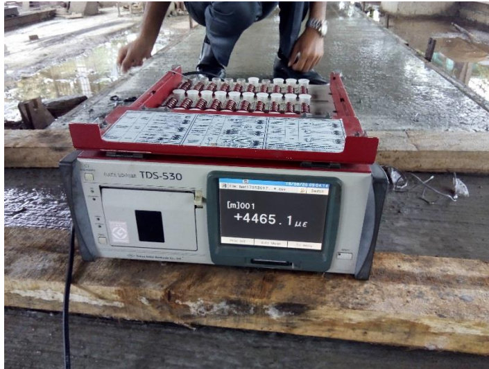
Figure 5.3.3 – Record data logger readings before releasing the strands
