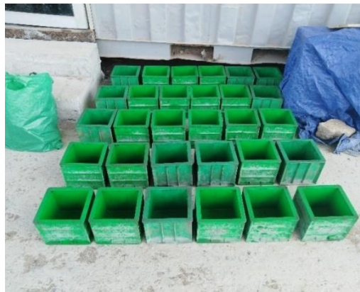
Figure 3-9 Preparation of moulds arrangement for splitting shear test
