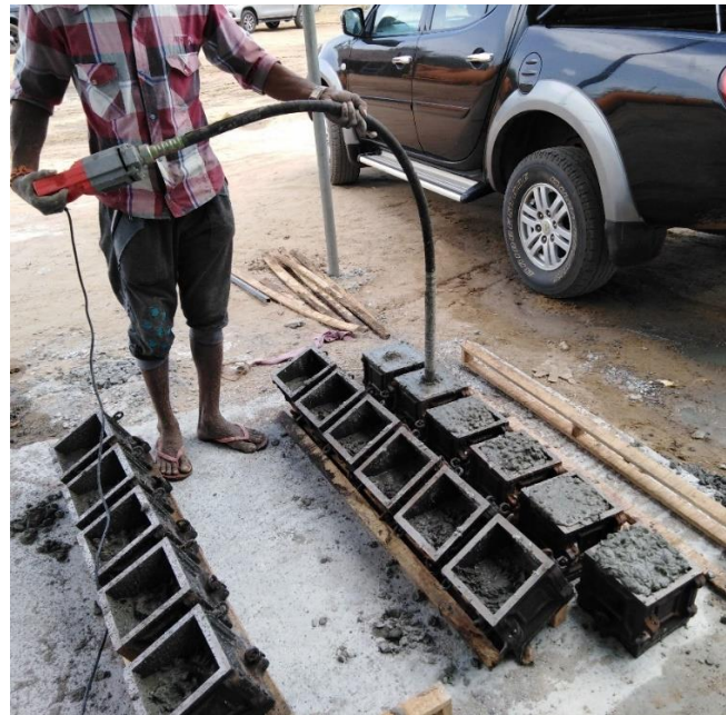
Figure 3-17 Compaction of 2 nd layer
