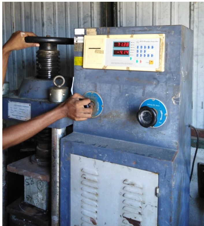
Figure 3-31 Testing of splitting tensile strength
