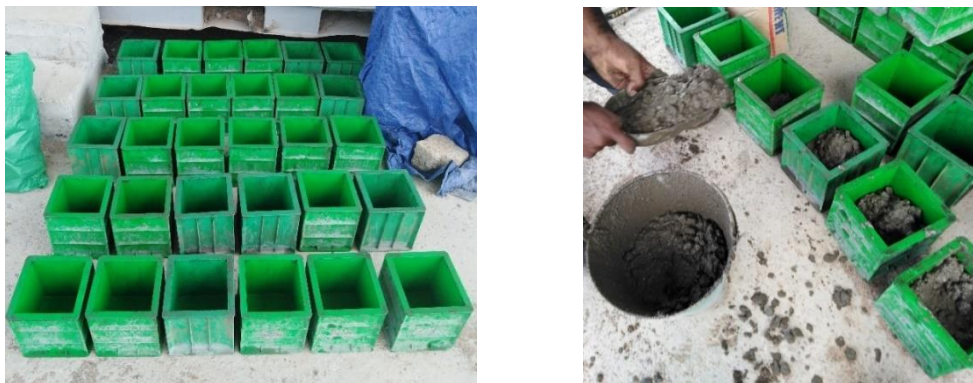
Figure 3-22 Casting 1 st layer for cold joint with horizontal plane
