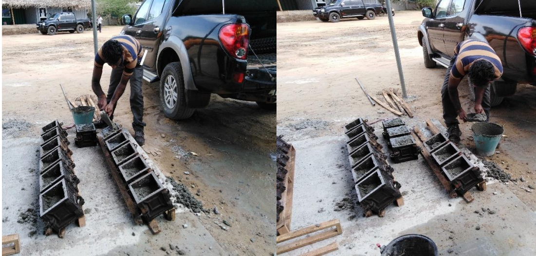
Figure 3-16 Casting 2 nd layer for zero delay time
