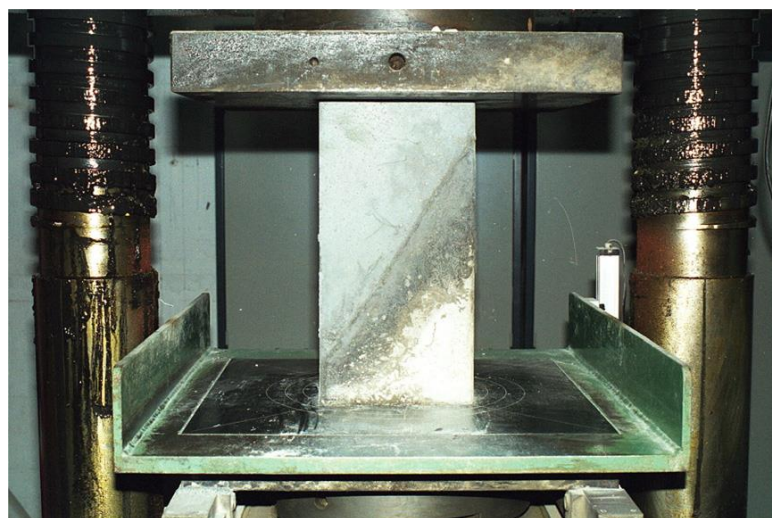
Figure 2-17 Slant shear test (Santos et al., 2006)
