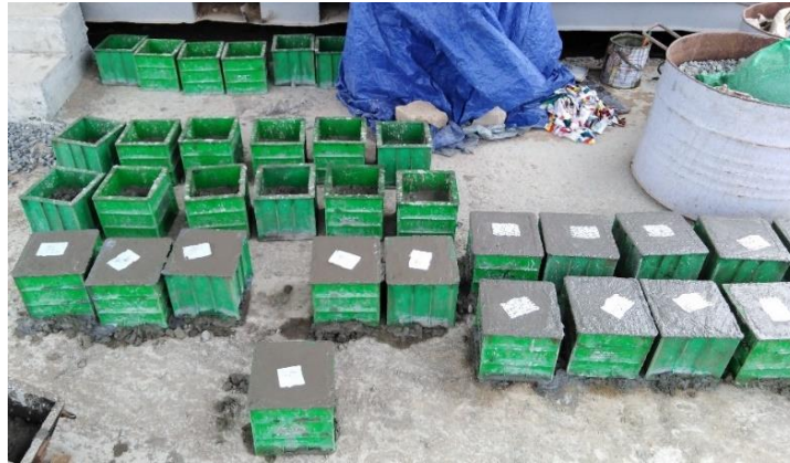
Figure 3-24 Casting 2 nd layer with delay time
