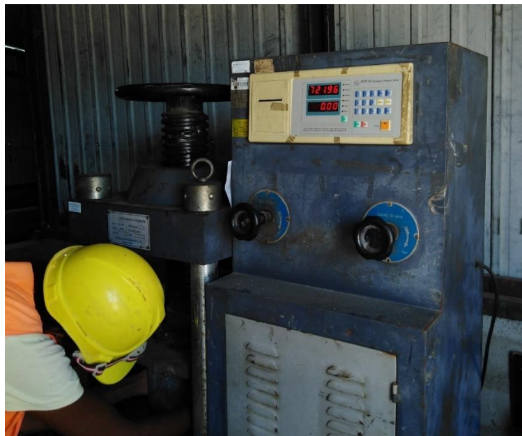
Figure 3-29 Testing of compressive strength
