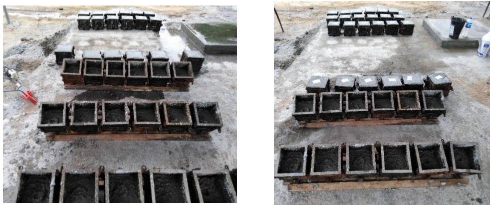
Figure 3-20 2 nd layer cast after 2hours (L) and 3hours (R) delay time, respectively
