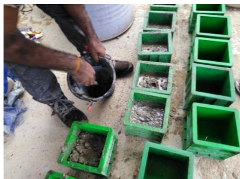
Figure 3-23 Applying bonding agent
