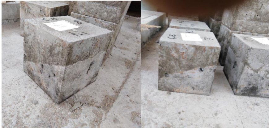
Figure 3-26 Cold joint with 20-degree plane
