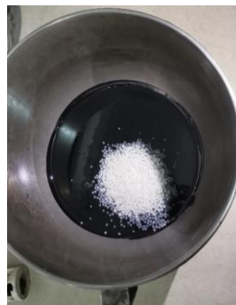
Figure 3.9 Sasobit Mixing with 60/70 Bitumen
