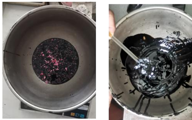
Figure 4.7 LDPE Mixing with Sasobit-modified Bitumen mixture
