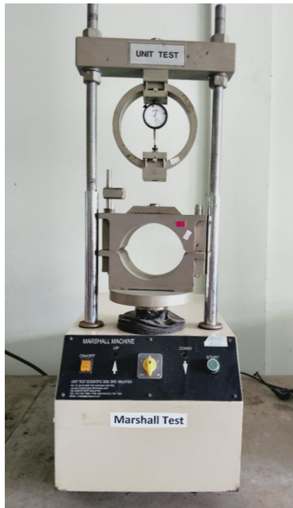
Figure 3.7 Marshall Stability & Flow Testing Machine
