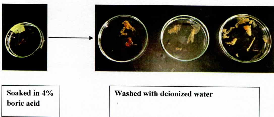
Figure 4.48: cross-linking of phytase enzyme encapsulated nanofibers with boric acid.
