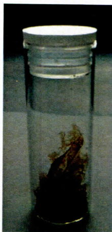
Figure 4.50: Cross-linked vacuum dried phytase enzyme encapsulated nanofibers
