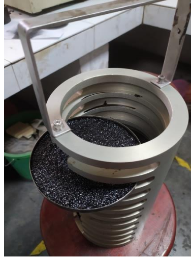
Figure 3.21: Aged bitumen in pans
