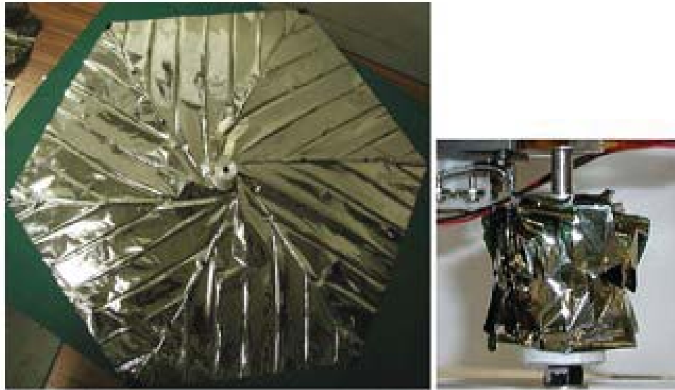
Fig. 6.1: Spiral folding pattern membrane model deployed and wrapped state [18]
