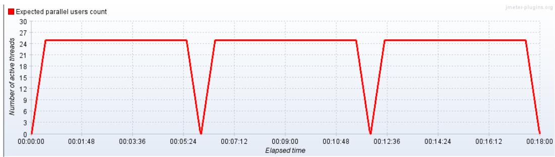
Fig 1.8: High growth-static-high shrink on-off with no interval workload pattern
