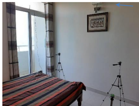
Figure 3.25: Data collection in a bedroom in Case study 2 utilizing Hobo data loggers
