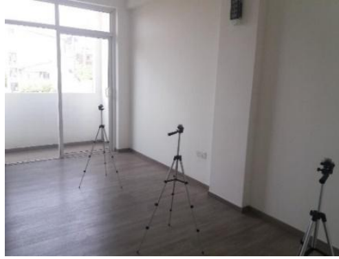
Figure 3.19: Data collection in a bedroom in Case study 1 utilizing Hobo data loggers
