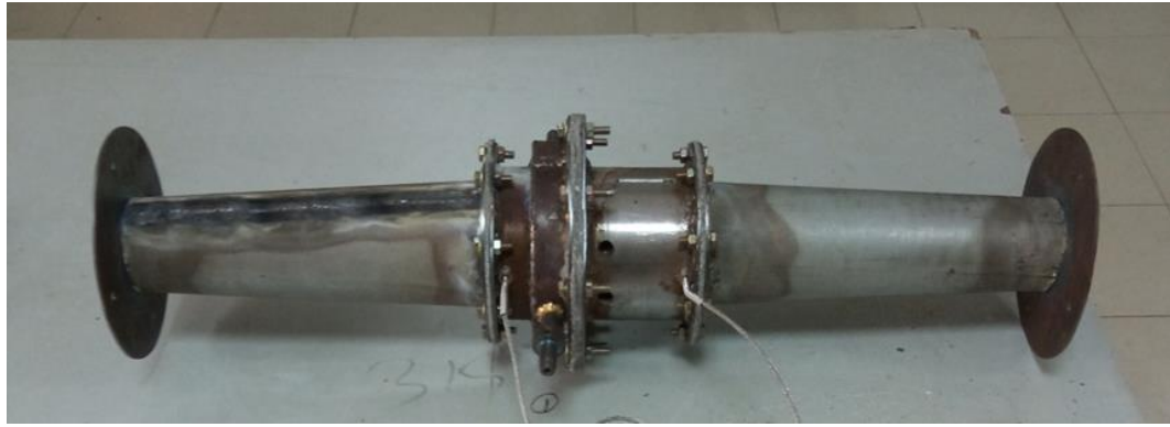
Figure 3.8 3D model and fabricated thermoacoustic core assembly
