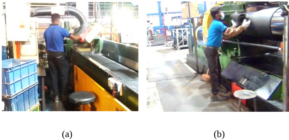
Figure 4-3: (a) Mixer operation process, (b) Rubber mill operation process
