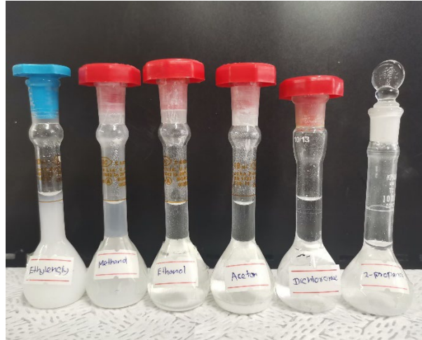
Fig. 2.5: The solubility of ZnO powder in various alcohols
