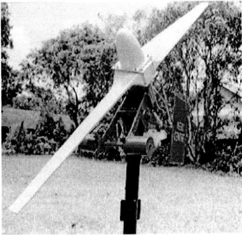
Figure 2.3: Tilt-up rotor passive control system
