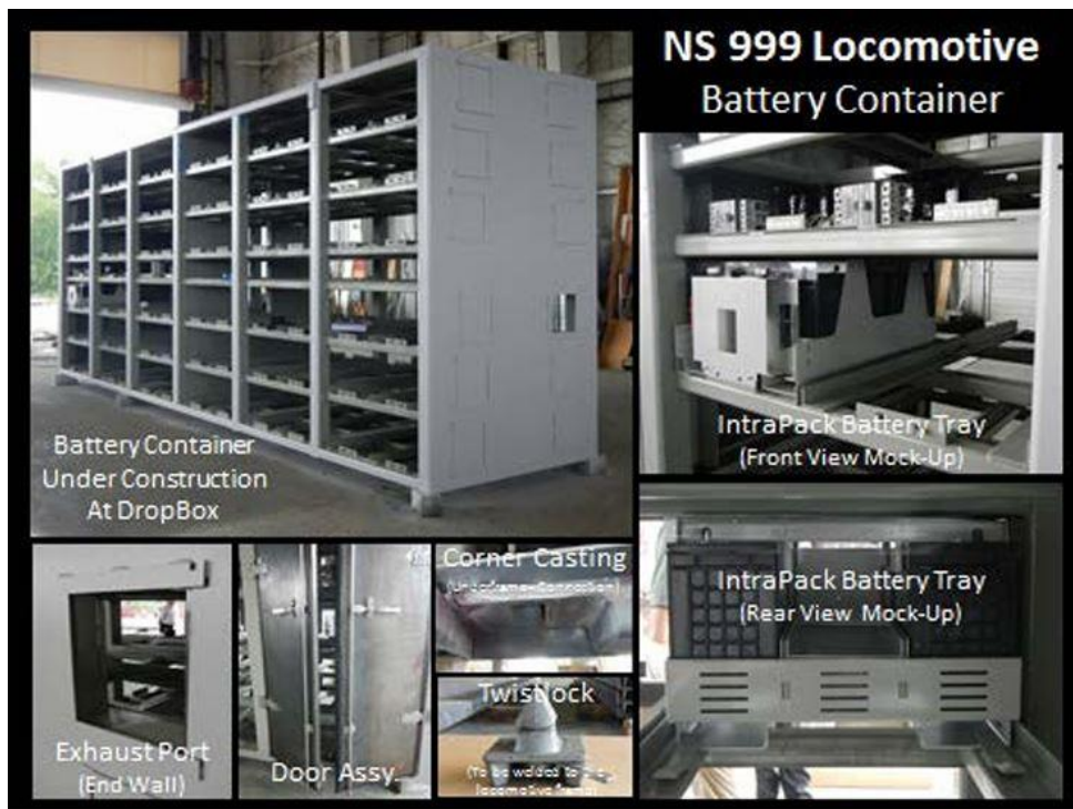
Figure 2.7: Battery ISO container for the NS 999, produced by DropBox, Inc. [29]
