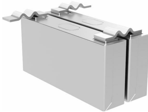
Figure 2.11: Interconnection layout for prismatic battery cells [35]
