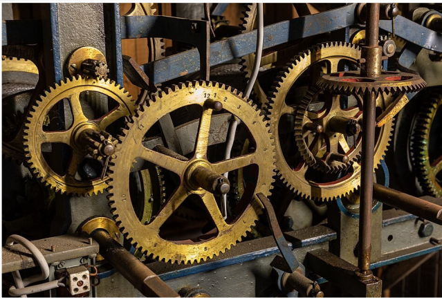
Fig. 4. Gear train of the clockwork in the Heilig-Kreuz-Kirche, Dülmen, Germany [12]. Image: Dietmar Rabich, CC BY-SA 4.0.
