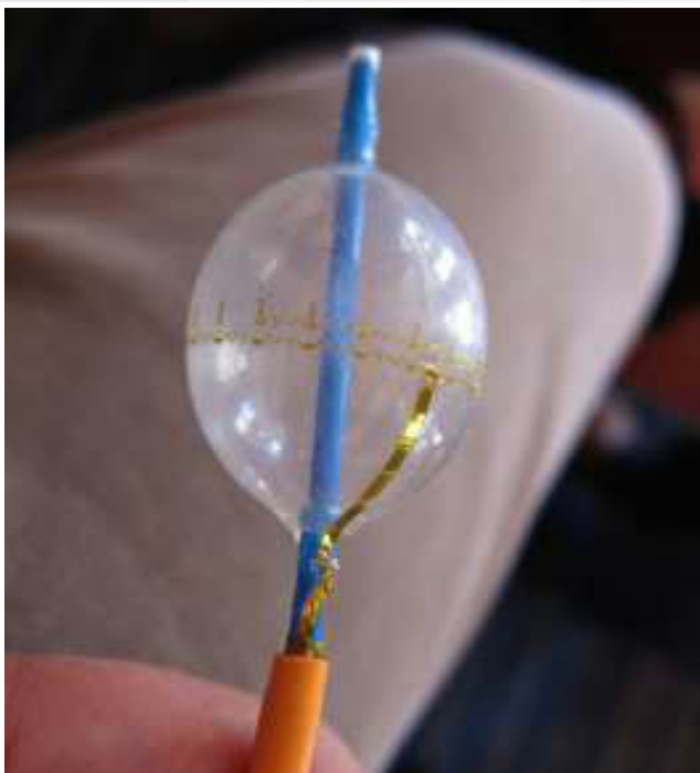
Fig. 3. A stretchable electronic circuit wrapped around a cardiac balloon catheter [19]. Licensed under CC BY 2.0.
