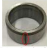
(b) Inner bearing fault
