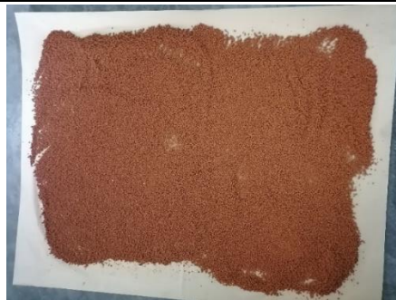
Figure 3. 14 Aggregate spread on paper towel to achieve saturated surface dry condition
