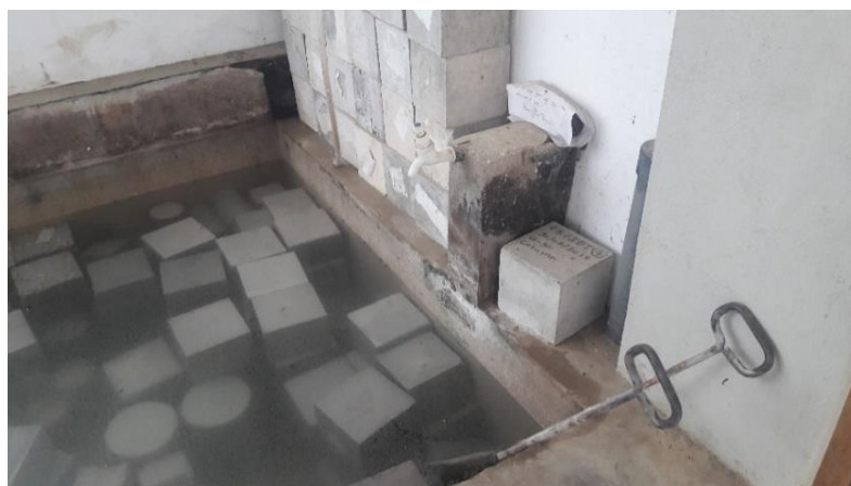
Figure 3. 16 External curing of concrete
