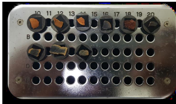
Figure 3. 7 Arrangement of sample for SEM analysis
