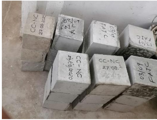
Figure 3.17 Cubes are left outside for no curing purposes
