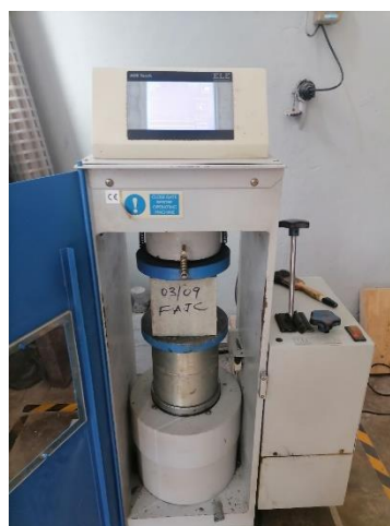
Figure 3.19 Compressive strength test apparatus for concrete
