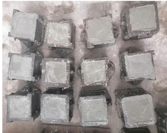
Figure 3. 15 Casted concrete cubes
