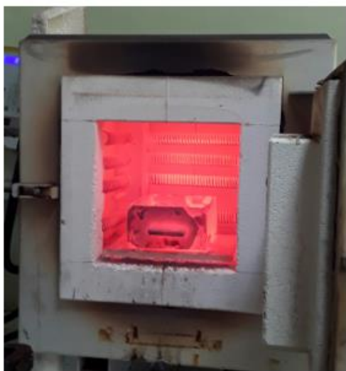
Figure 3. 6 Sintering of fly ash sticks in laboratory kiln
