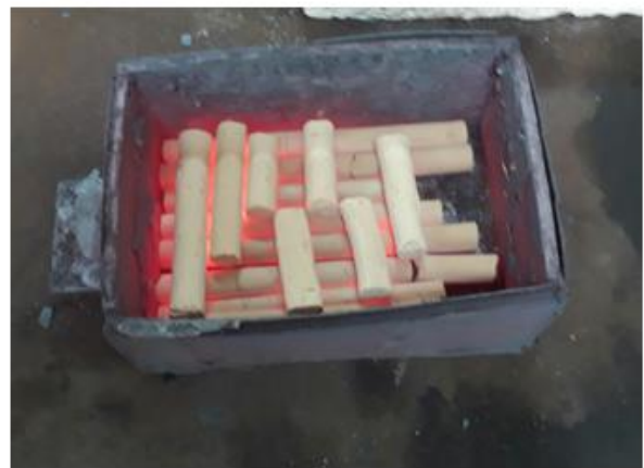
Figure 3. 6 Sintering of fly ash sticks in laboratory kiln
