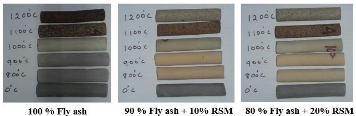
Figure 4. 3 Colour variation of sintered cylindrical samples
