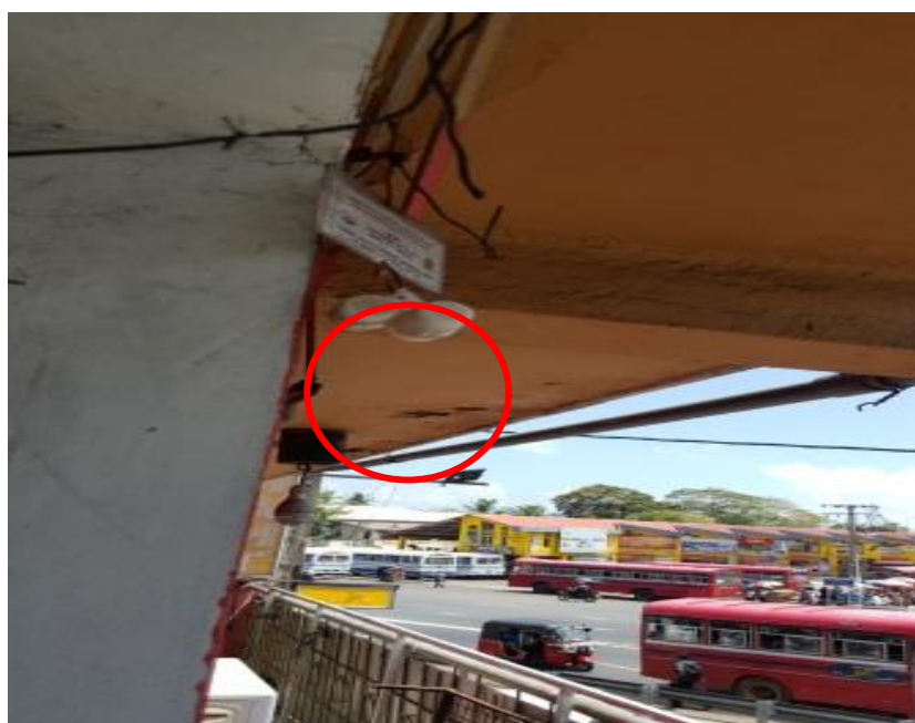
Figure 3-4: Passive samplers installed at Kalutara Municipal council
