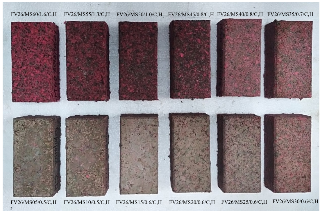
Figure 4.16: Surface texture of paving blocks belonged to different mix proportions
