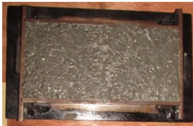
(c) Cast tile samples in two gang square mould
