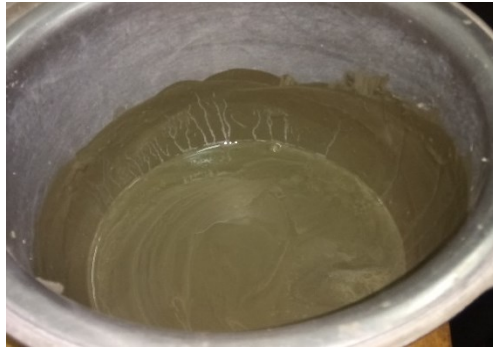
(a) Viscous cement slurry (Cement + admixture + water)
