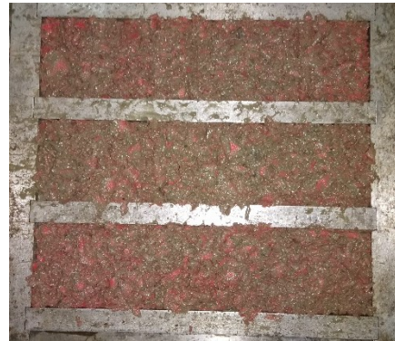
(e) Cast prism specimens ready for curing
