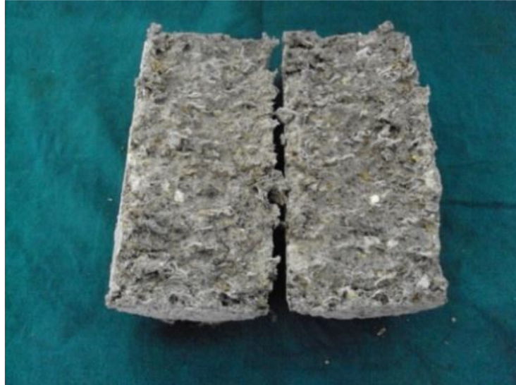
Figure 2.4: Split section of waste cloth concrete [9]
