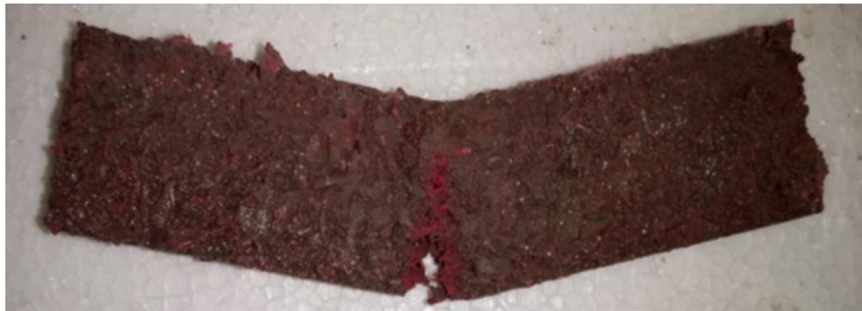
Figure 4.13: Failure pattern under flexural load
