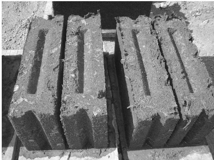
Figure 2.5: Surface appearance of fabric incorporated cement block [10]
