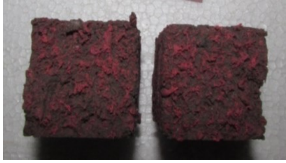
Figure 4.14: Fracture surface under flexural load
