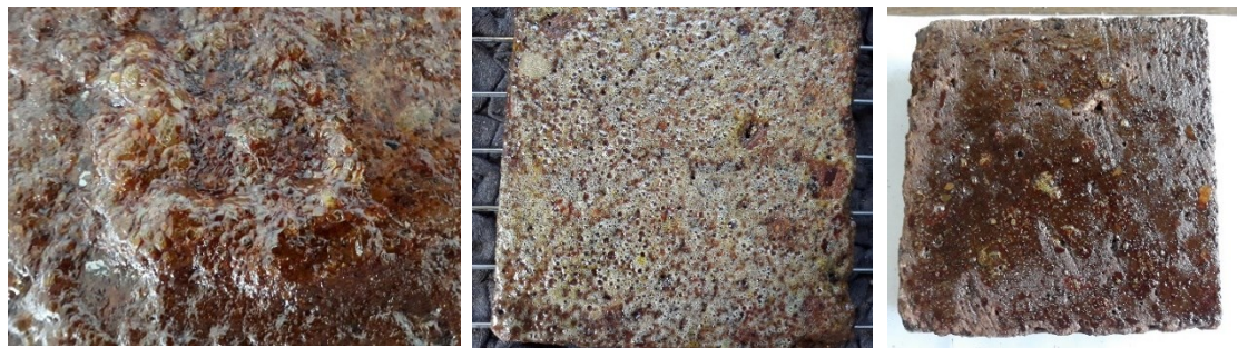
Figure 5-12: Surface appearance after heating due to over-application and overheating
