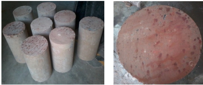
Figure 3-23: Top surface of cylindrical specimens prepared for testing
