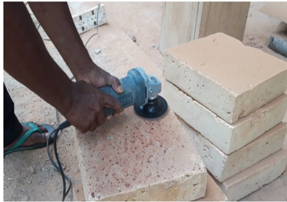
Figure 5-2: Process of surface preparation by grinding and sandpapering
