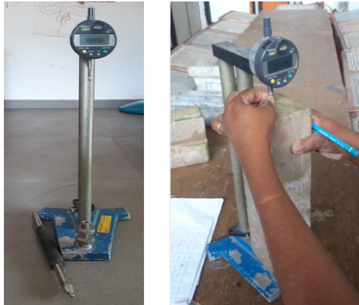
Figure 3-29: Apparatus used to measurement of length change
