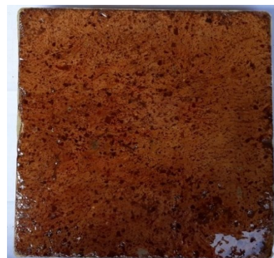
Figure 5-10: Surface appearance after applying resin but before heating
