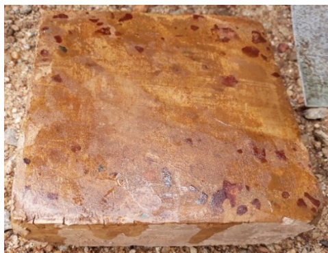
Figure 5-10: Surface appearance after applying resin but before heating
