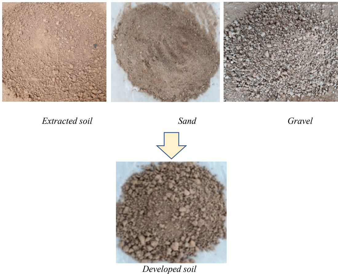
Figure 3-8: Preparation of soil to the required particle size distribution and developed soil
