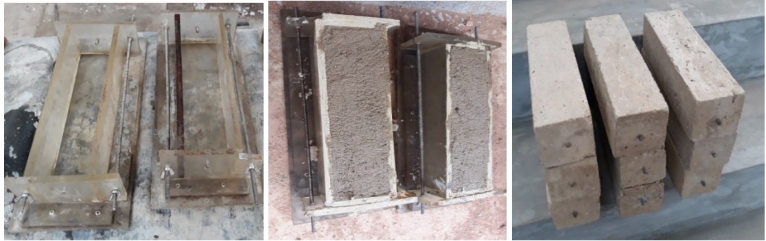
Figure 3-28: Moulds and specimens for shrinkage test
