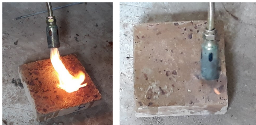
Figure 5-15: The heat application process
