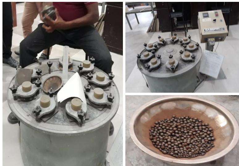
Figure 5-30: Abrasion test procedure in the laboratory at Meepe Lanka Tile factory
