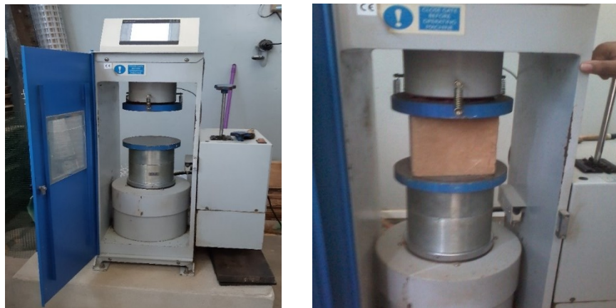
Figure 3-11: Compressive strength testing procedure
