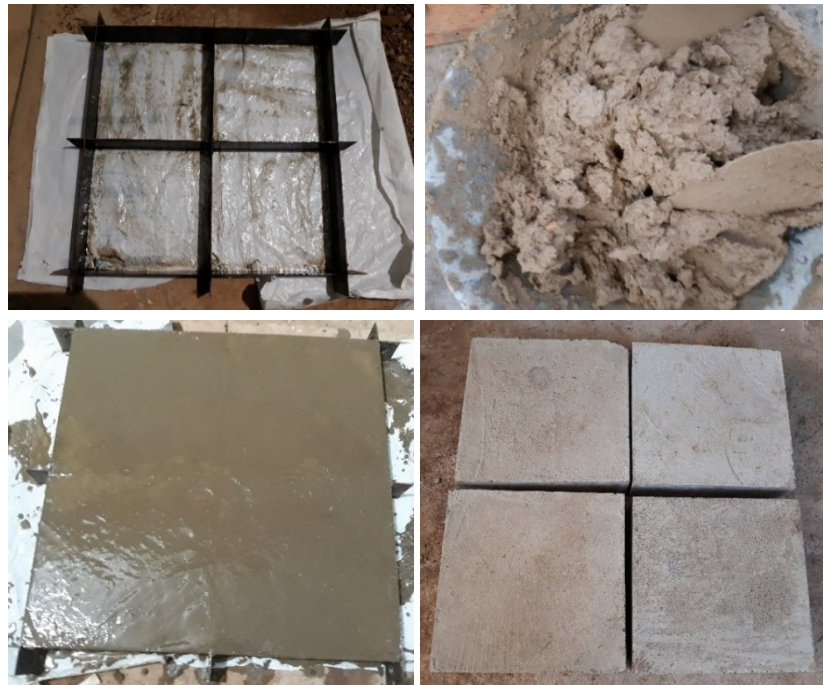
Figure 5-1: The process of casting floor samples and prepared floor samples
