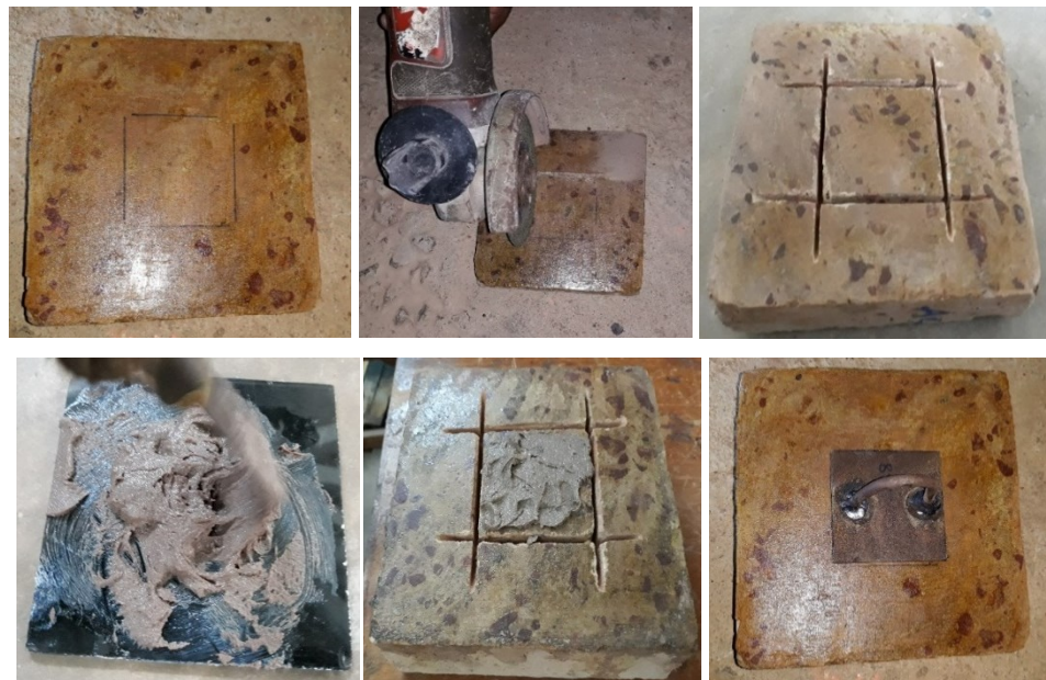
Figure 5-19: Preparation of floor samples for Pull-off test
