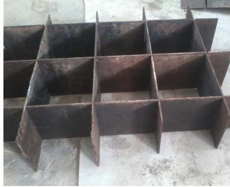
Figure 3-9: Steel mould used for specimen casting
