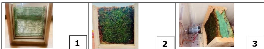
Figure 3, Actual setups (1) - Filter configuration including panels, (2) the front panel installed with moss (3) filter installation in the experiment chamber
