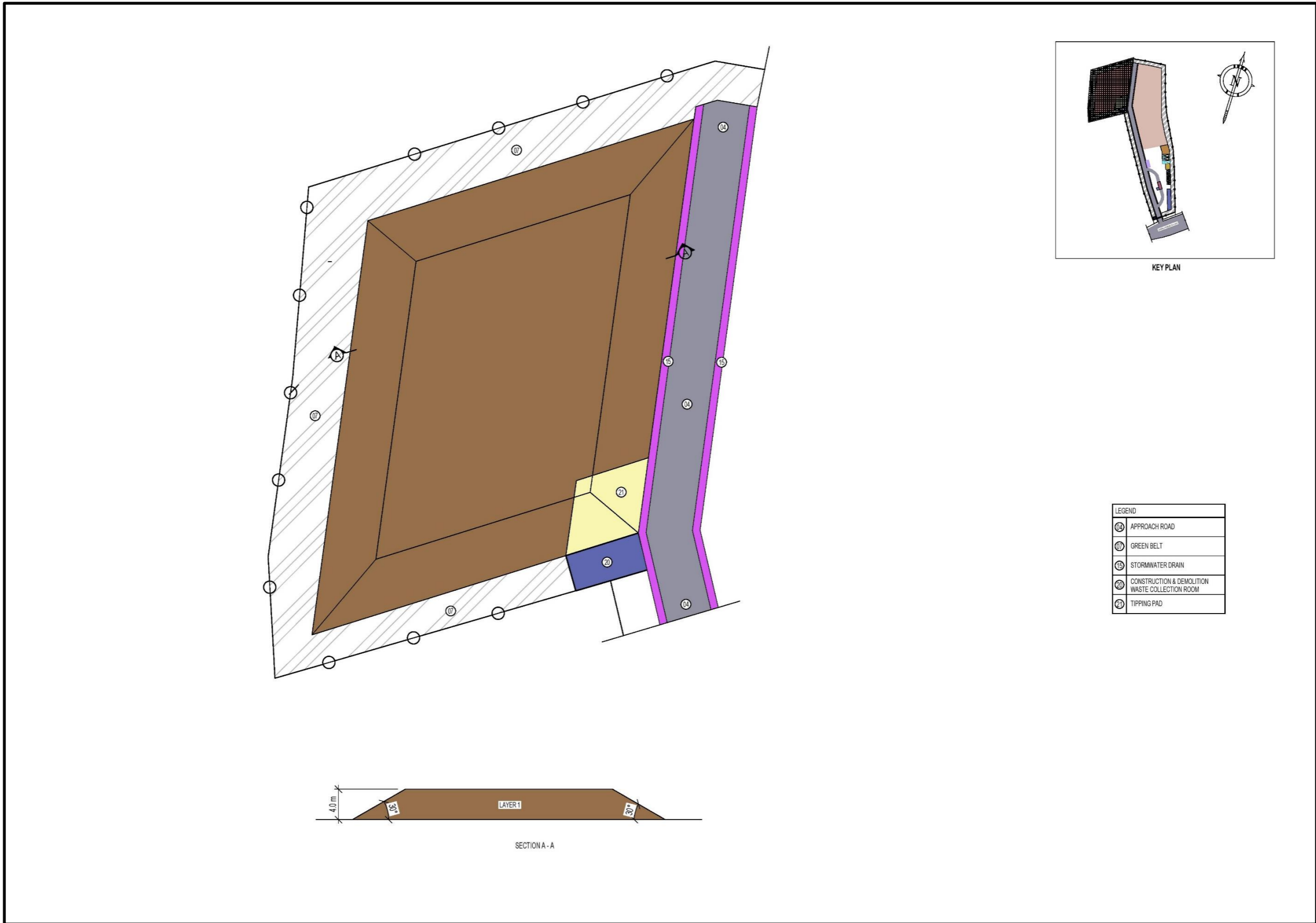
Figure A.9: Layout of the controlled landfill after the completion of layer-1
