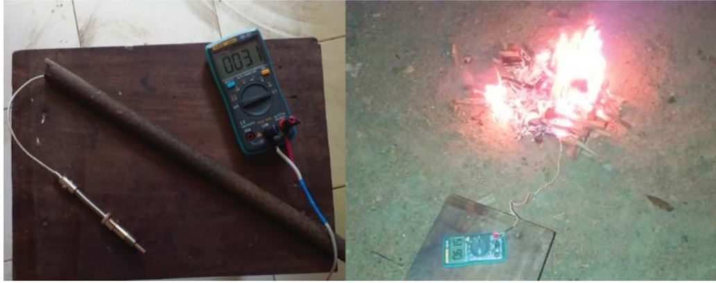
Fig. 4.3: Thermocouple for actual temperature measurement of the fire
