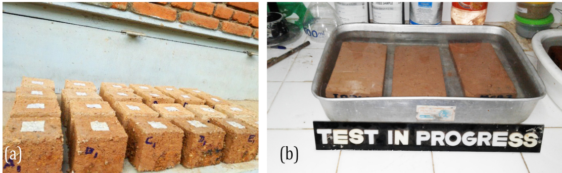
Fig. 4.32 NRL stabilized blocks are immersed in water for the study
