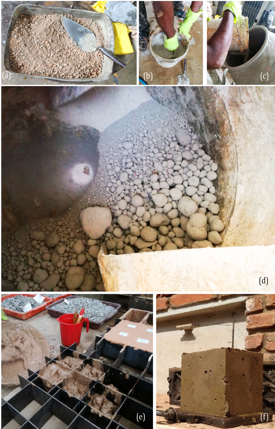
Fig. 5.3 Casted geopolymer blocks
