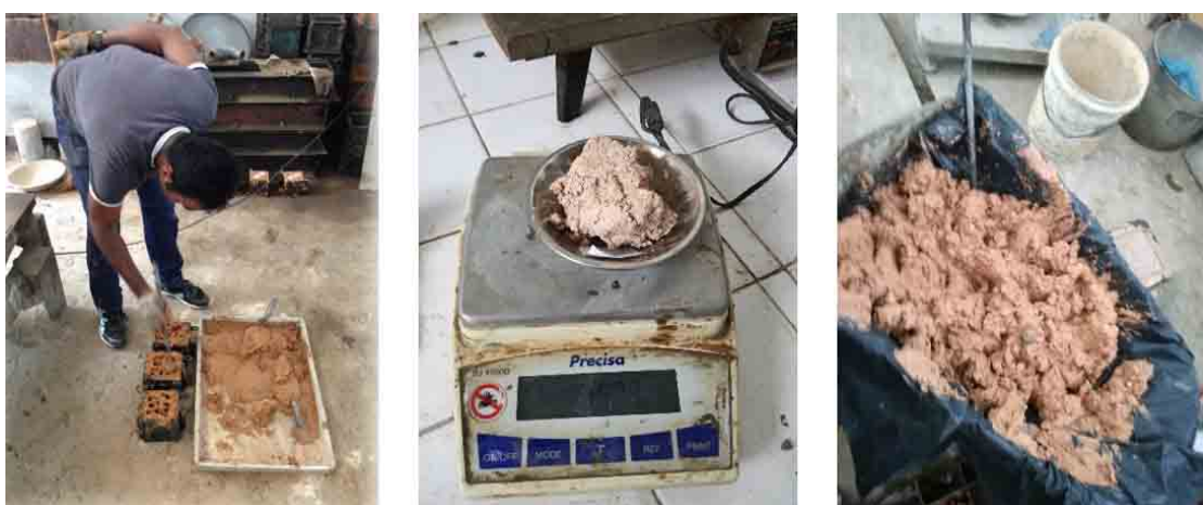
Fig. 3.2 Blind mixes with different alternative stabilizers and mud concrete mix
