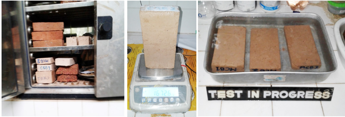
Fig. 3.10 Water absorption test
