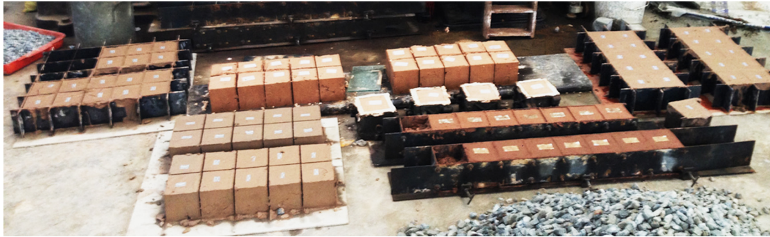
Fig. 4.1 Different mix design blocks prior to test
