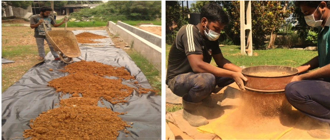
Fig. 3.4 Sieving soil into three different soil particle combination
