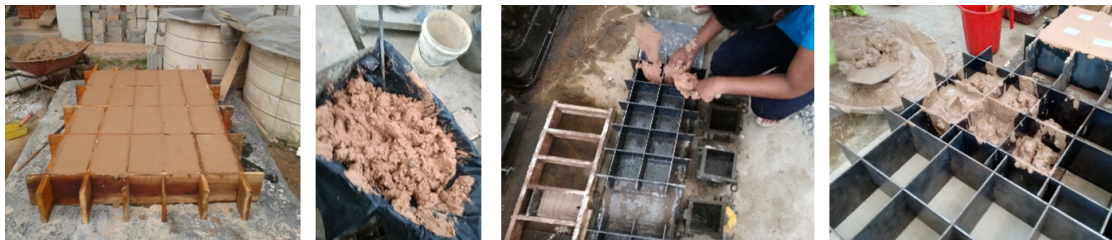
Fig. 3.7 Testing block manufacturing and workability of soil
