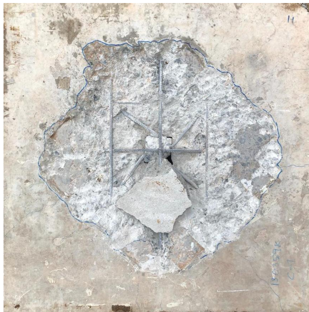
Figure 3.17. Crack Pattern of Control Specimen
