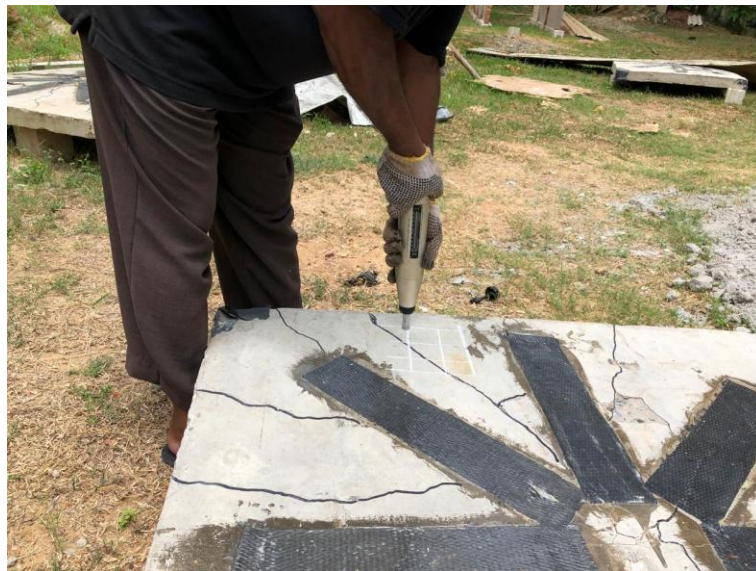
Figure 3. 3. Re-bounce Hammer Testing
