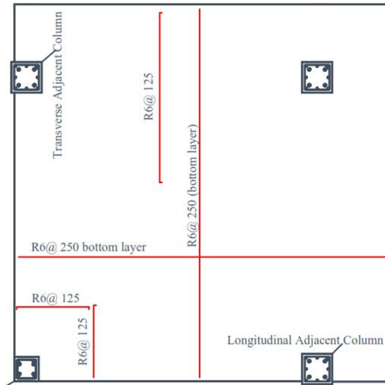
Figure 2.2. Reinforcement Arrangement (Kai et al., 2013)
