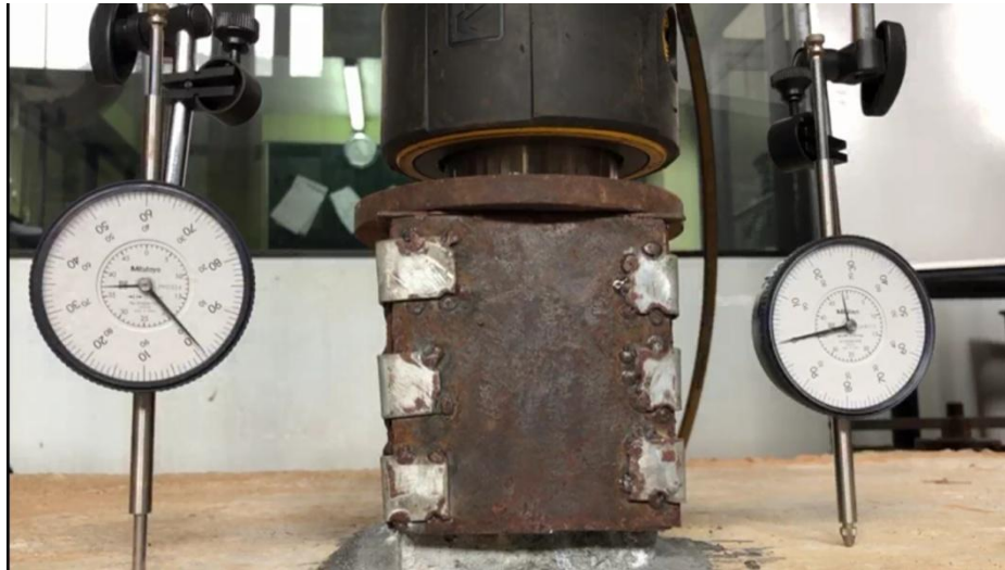
Figure 3.14. Dial Gauge Arrangement
