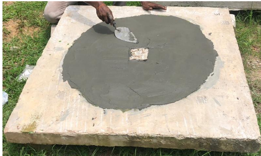
Figure 3. 5. Preparation of Specimens without Epoxy Bond
