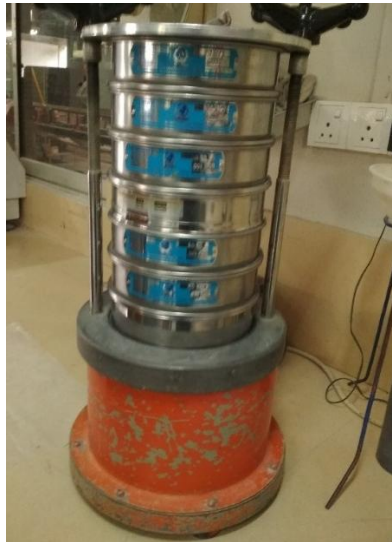
Figure 3.6: Used sieves and ceramic waste inside a sieve
