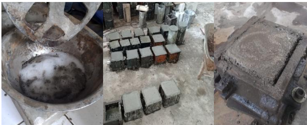
Figure 3.12: Steps for preparing concrete cube samples
