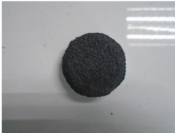
Figure 5.1-Circular sample cut from the glove palm
