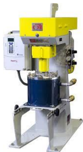
Figure 4.5- Vertical Glass pebble mill
