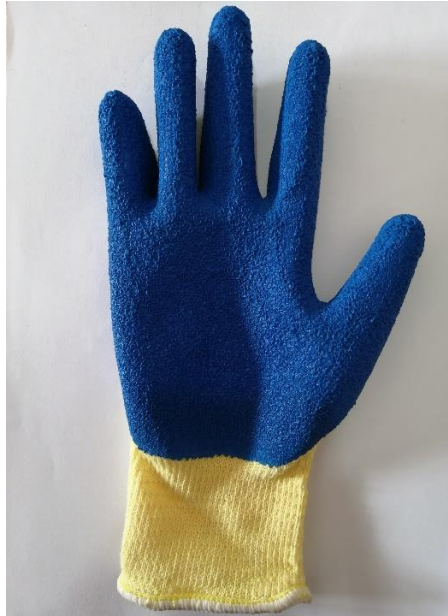
Figure 7.3-Experiment-03, Precipitate silica-based glove sample
