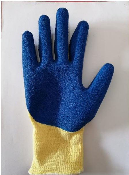
Figure 7.4-Experiment-03, Fume silica-based glove sample
