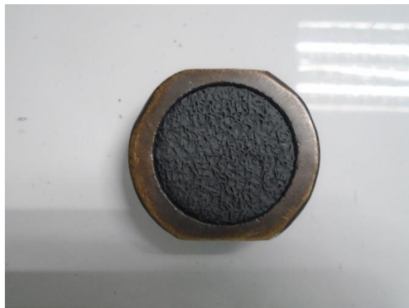
Figure 5.1-Circular sample cut from the glove palm
