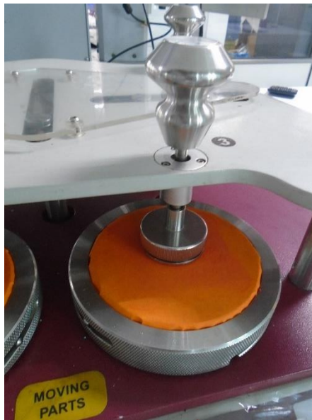
Figure 5.4-Fix the sample holder to Martindale abrasion tester
