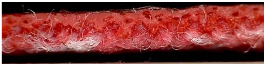
Figure 7.27-Cross Section-Calcium carbonated filler loaded glove sample
