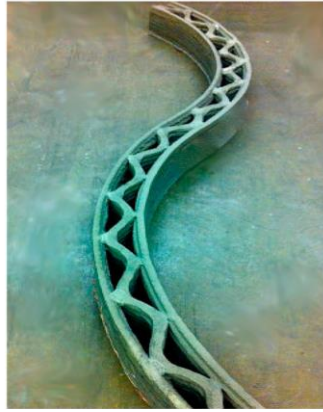
Figure 2.2: Concrete printing (Bos, et al., 2016)
