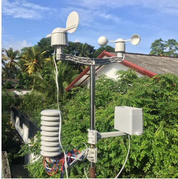
Figure 5.2: Weather Data Capturing Unit
