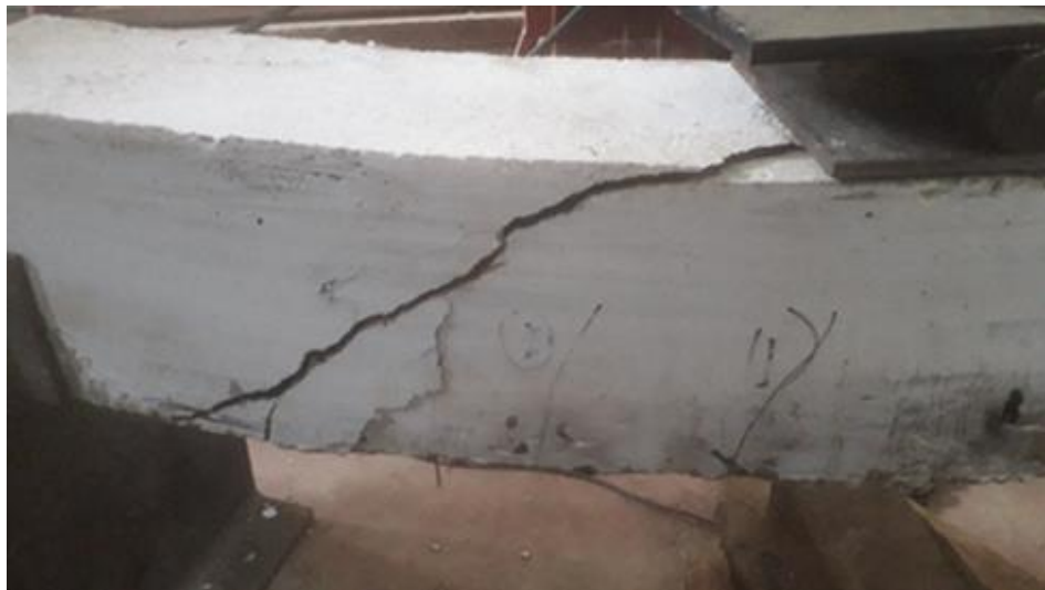
Figure 37: Shear failure of a control beam
