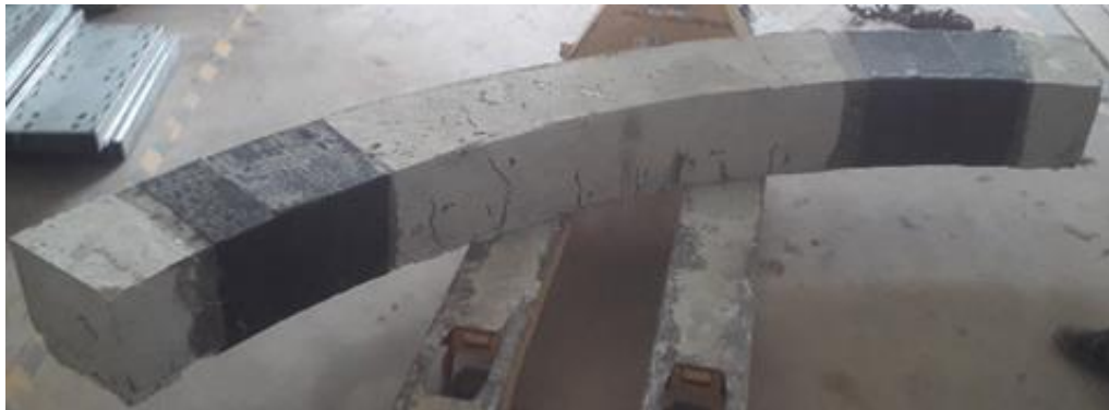
Figure 41: Flexural cracks at mid-span
