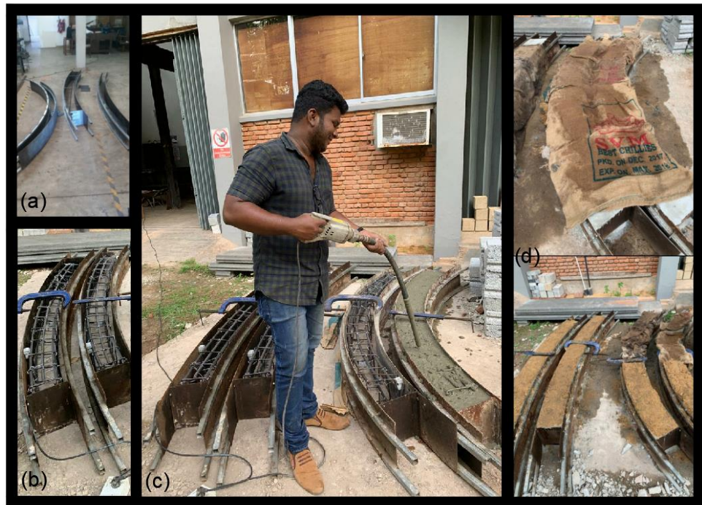
Figure 33: Specimen preparation (a) Custom made steel shuttering for formwork (b) Steel reinforcement cages placed in steel shuttering and cover maintained with cover blocks (c) Concreting and compacting (d) Curing of cast specimens using sand and gunny bags.
