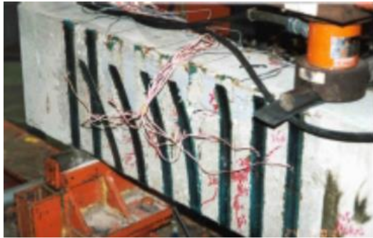
Figure 25: FRP debonding failure of a U jacketed RC beam (Teng et al., 2001)
