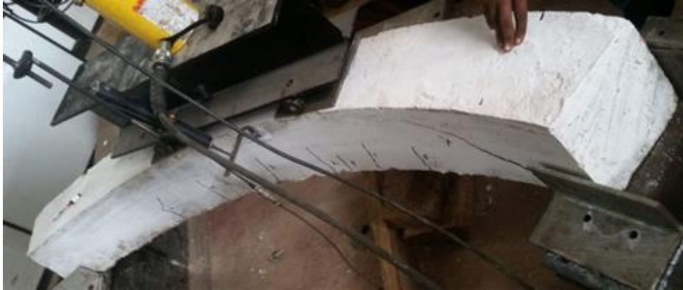
Figure 36: Cracks in a failed control beam
