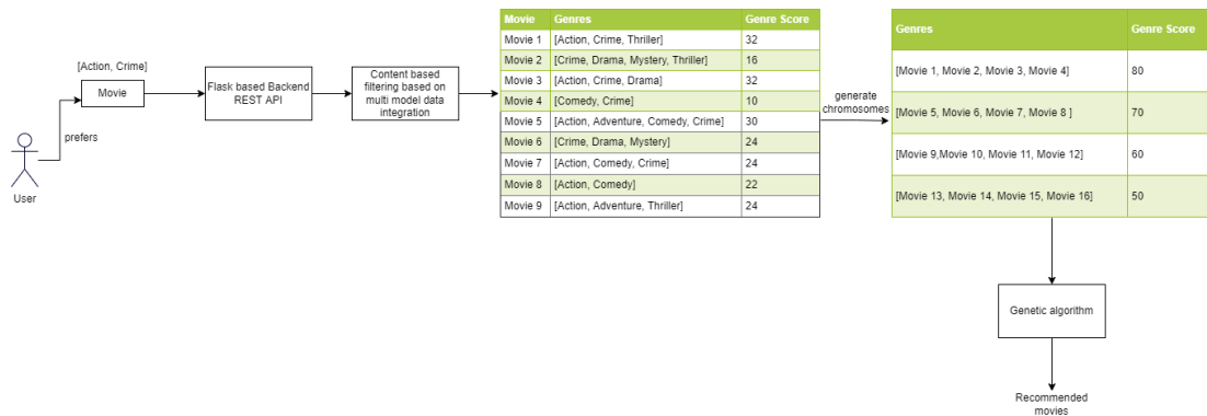
Figure 6.2.5. 1 Architecture of evolutionary computing-based approach
