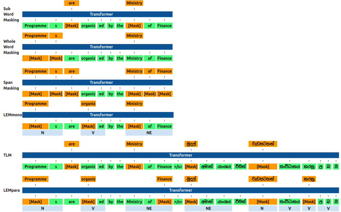
Figure 5.2: A comparison of existing masking strategies is presented using an example from the English-Sinhala language pair. Sub-word masking, Whole Word masking, span masking, and LEM_{mono} exclusively utilize monolingual sentences during masking. In contrast, TLM and LEM_{para} apply masking on concatenated parallel sentences. Notably, in both LEM_{mono} and LEM_{para} , only a single token from the linguistic entity is masked.
