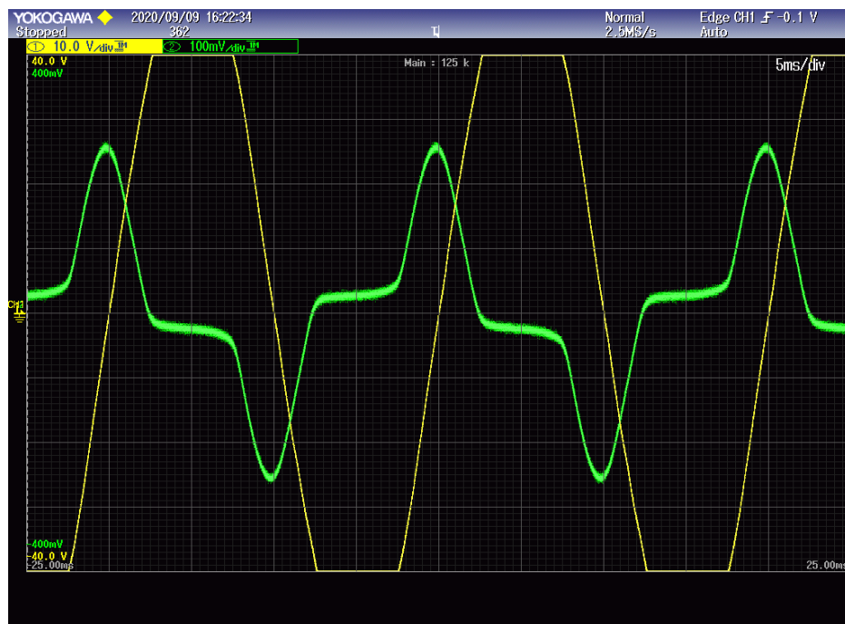
Figure 9: Single Phase Transformer - Rated Voltage Waveform (Yellow) and Current Waveform (Green) Plotted in Oscilloscope
