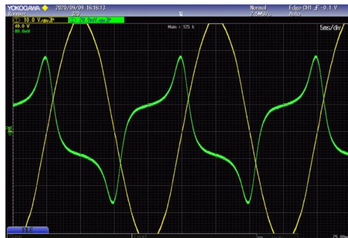
Figure 14: Single Phase Transformer - 75% of Rated Voltage Waveform (Yellow) and Current Waveform (Green) Plotted in Oscilloscope
