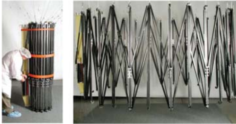
Fig. 2.1: Deployable mast that elements affixed by mechanical hinges
